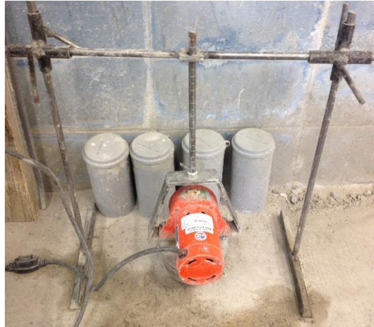
Figure 5. Adjustable steel frame to stabilize the VKelly apparatus
