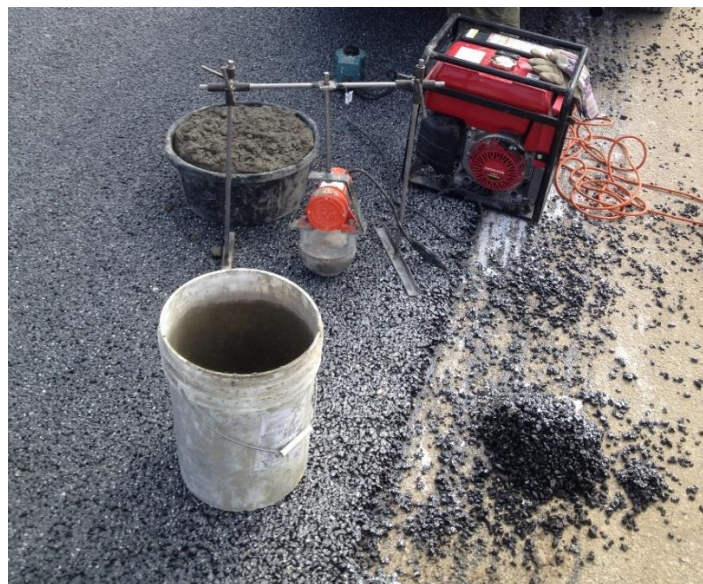
Figure 15. VKelly test conducted in the field
