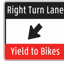
Sign Size: 36" x 30" Type height reduced from 4" to 3.5" Spacing reduced by -35 Negative contrast switched to Positive contrast
