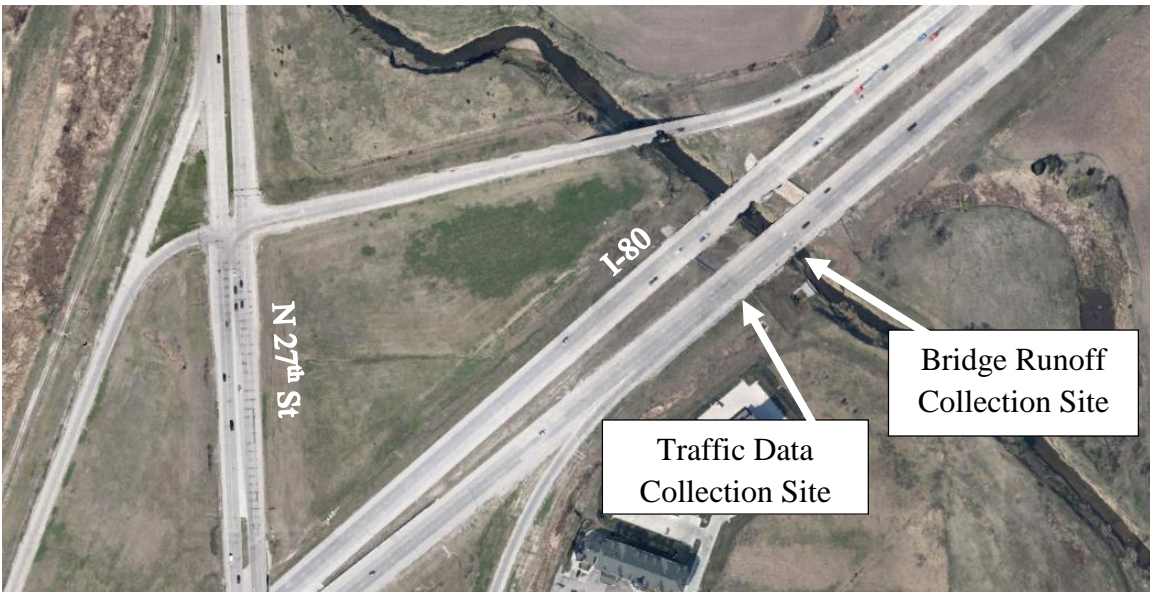
Figure 2.7 I-80 Little Salt Creek traffic data collection site
