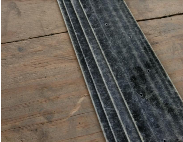
Figure 5 FRP Strips to be installed (VTrans 2014)
