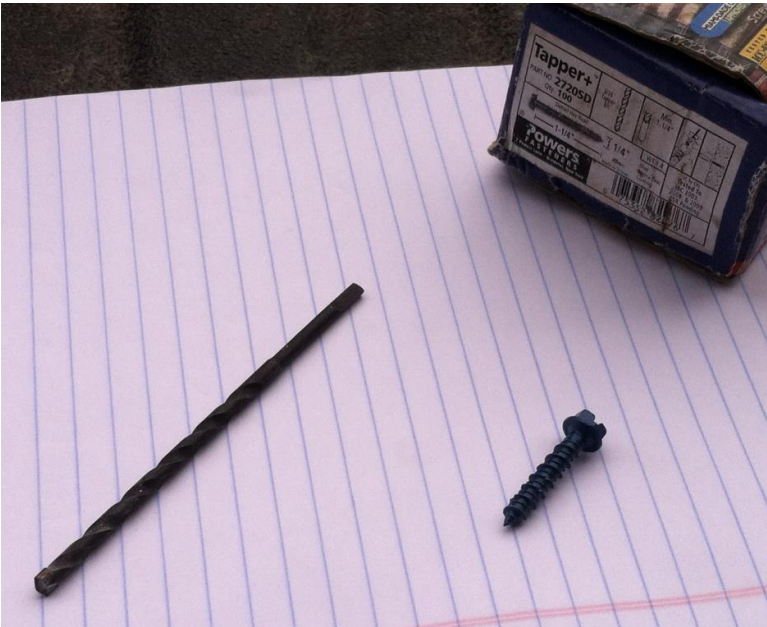
Figure 8 1/4" Tapper Plus® Coated Steel Concrete Screw (VTrans 2014)
