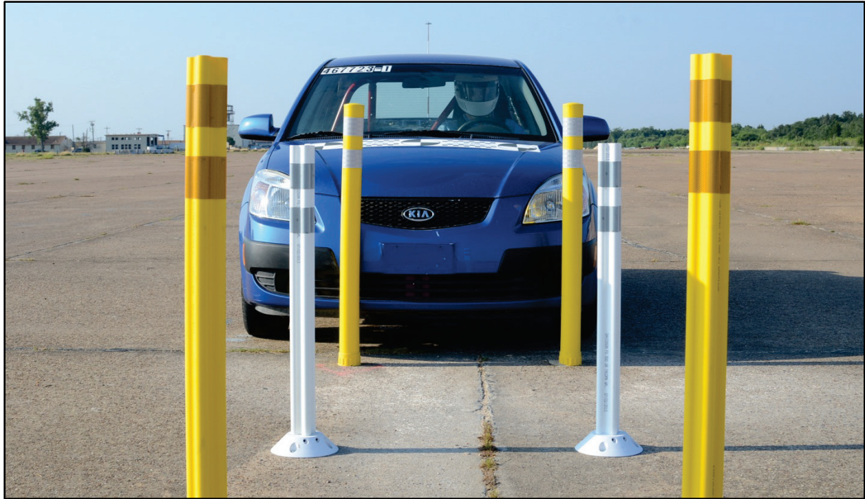
Figure 5.1. 1100C Impact Position before Testing.
