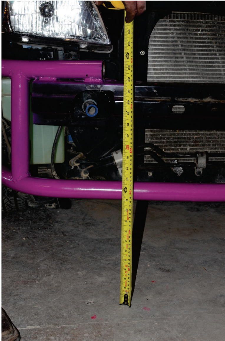
Figure 4.4. Modified Bumper Ground Clearance.
