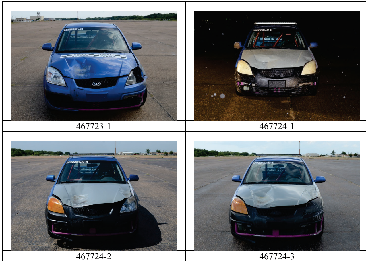
Figure 7.1. Bumper Shell Damage Comparison.
