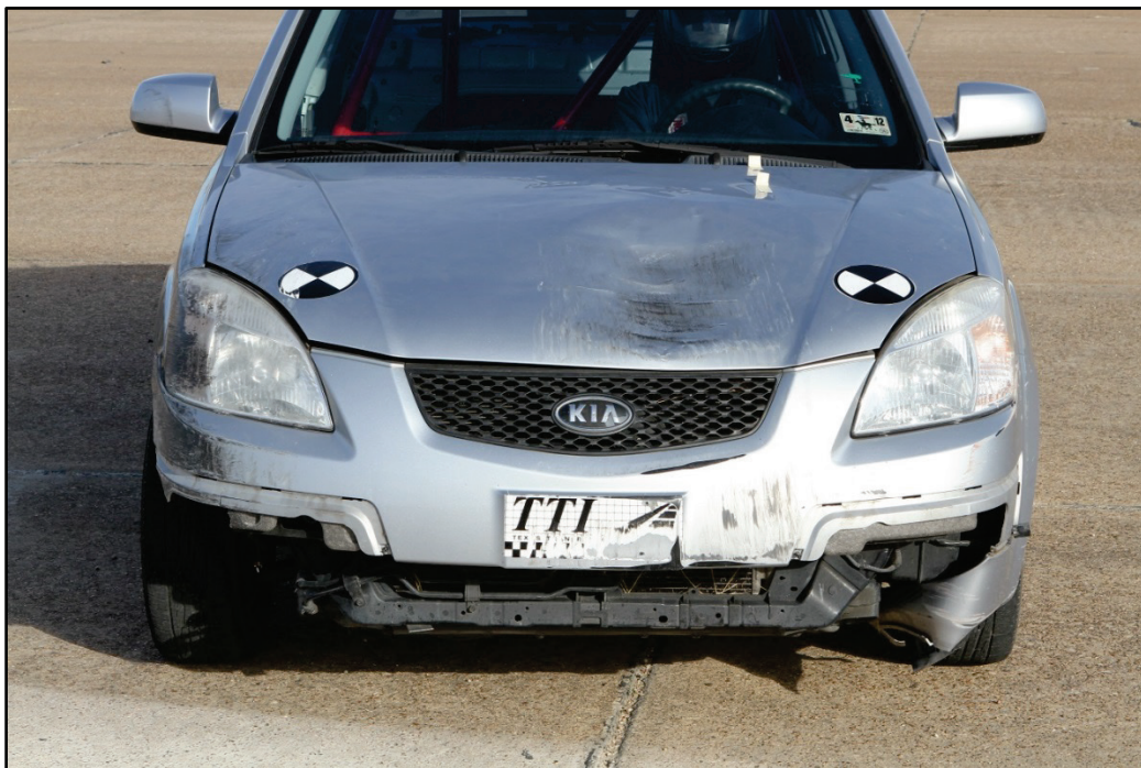
Figure 1.3. Kia Rio ( MASH Test Vehicle) after 100 Impacts.
