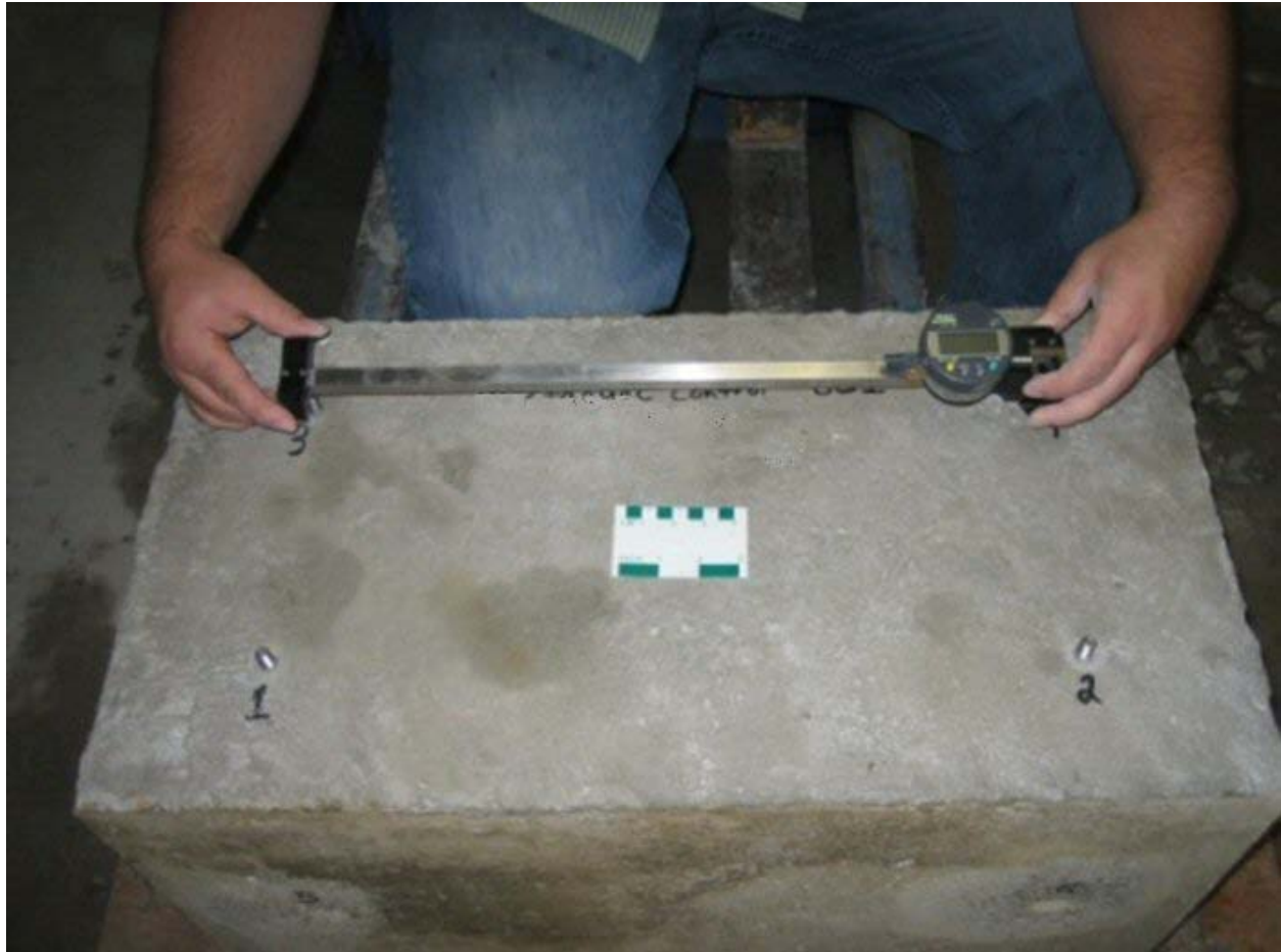
Figure 8. Length-Change Measurements Using a Demec-Type Gauge
