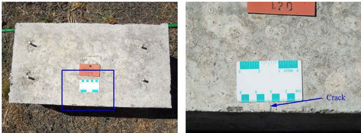
Figure 4. Photograph of Block 4 at 805 days (August 2013) (Photo on right is an enlargement of area in blue box on left)
