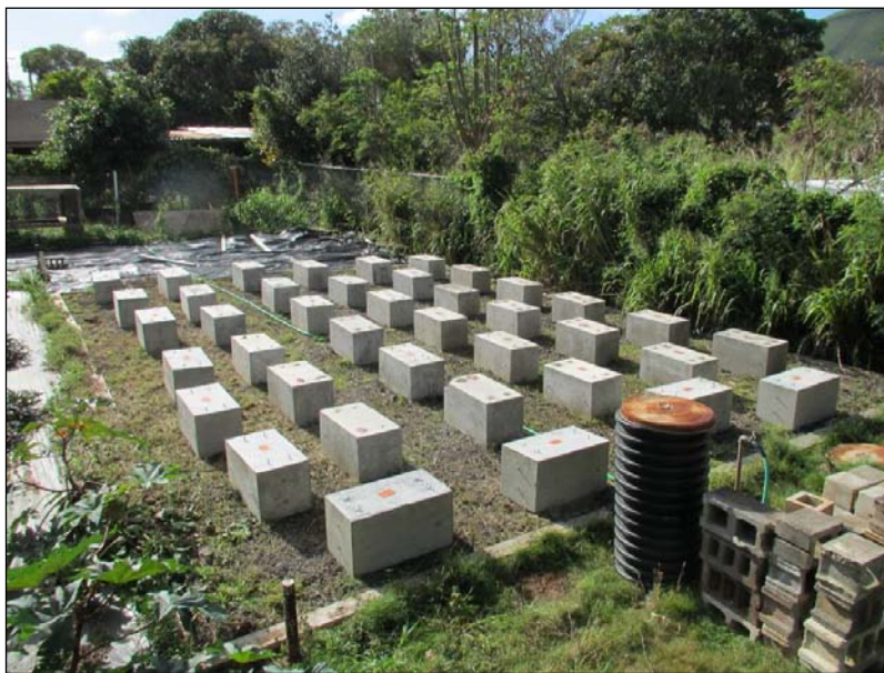
Figure 1. Completed Exposure Site at the University of Hawaii at Manoa, Hawaii (January 2013)
