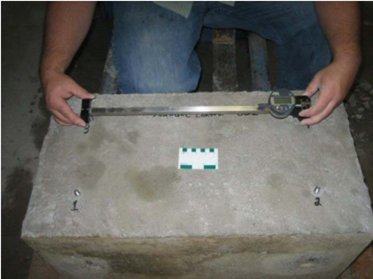
Figure 2. Length-Change Measurements Using a Demec-Type Gauge
