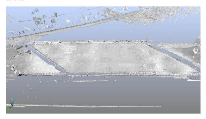
Figure 18 Point cloud for rebar surface
