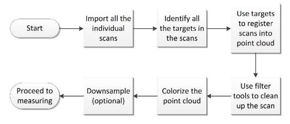
Figure 4 Bridge scans processing workflow
