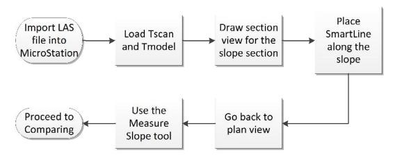
Figure 30 The slope measurement workflow
