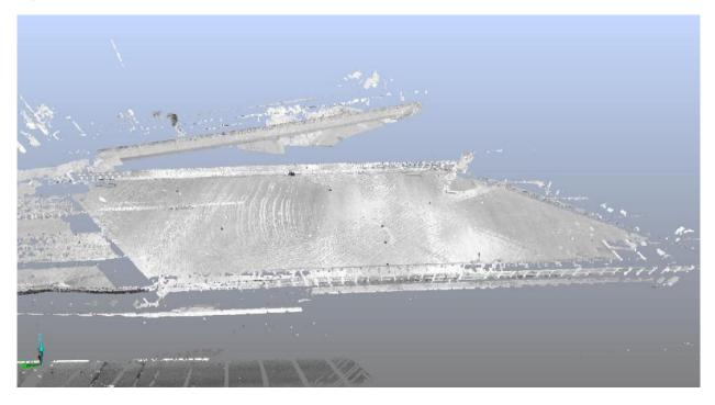
Figure 19 Point cloud for the concrete bridge surface
