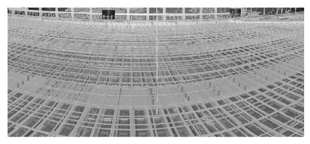
Figure 21 Bridge deck rebar in 3D point cloud
