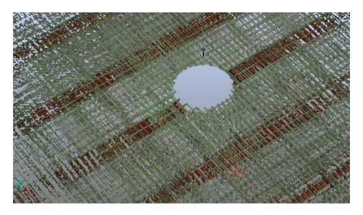
**Figure 16 Colorized Point Clouds for Rebar Cages**
