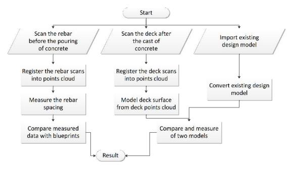
Figure 12 General workflow of bridge scan
