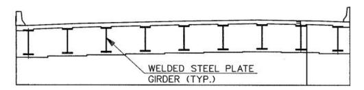
Figure 5 Typical bridge section
