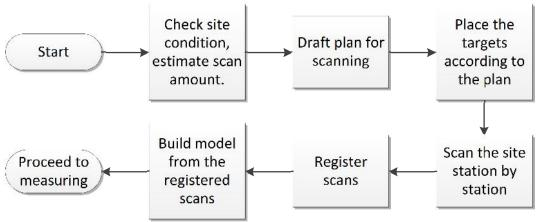
Figure 3 Typical Bridge Deck Scanning Workflow
