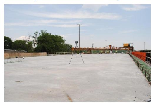
Figure 17 Scanning the concrete surface
