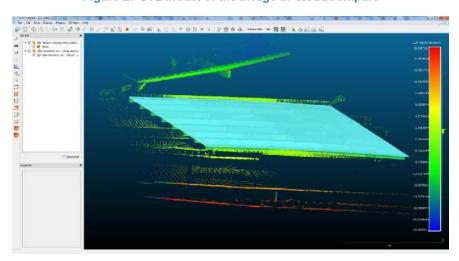
Figure 28 Difference between the aligned CAD and Point Cloud Data
