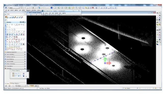
Figure 29 Measure the slope of bridge surface
