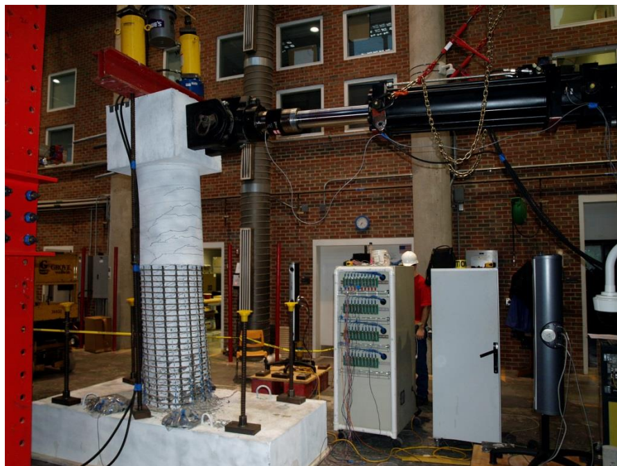
Figure 2.6 Specimen Under Lateral Deformation
