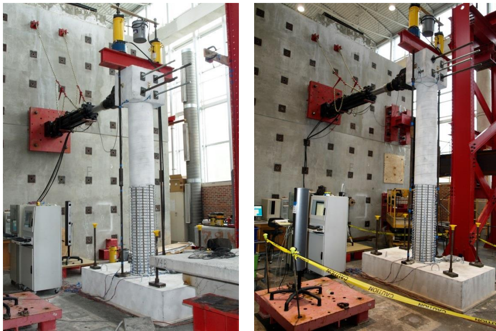
Figure 2.8 Test Setup for 11' and 13' Cantilever Length Specimens
