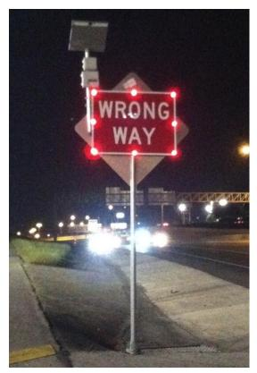
Figure 1. WRONG WAY Sign with Red Flashing LEDs around the Border.
