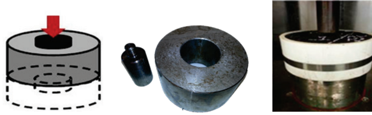
SPST Specimen Setup
