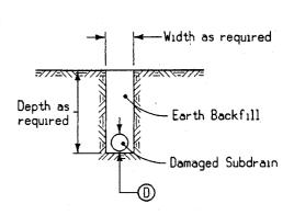
NOTE: Replacement of drainage tile shall be accomplished so as to cause the minimum of disturbance to existing field tile. The repaired drainage tile shall be left in a functional condition with special emphasis placed on maintaining existing flow line elevations.
