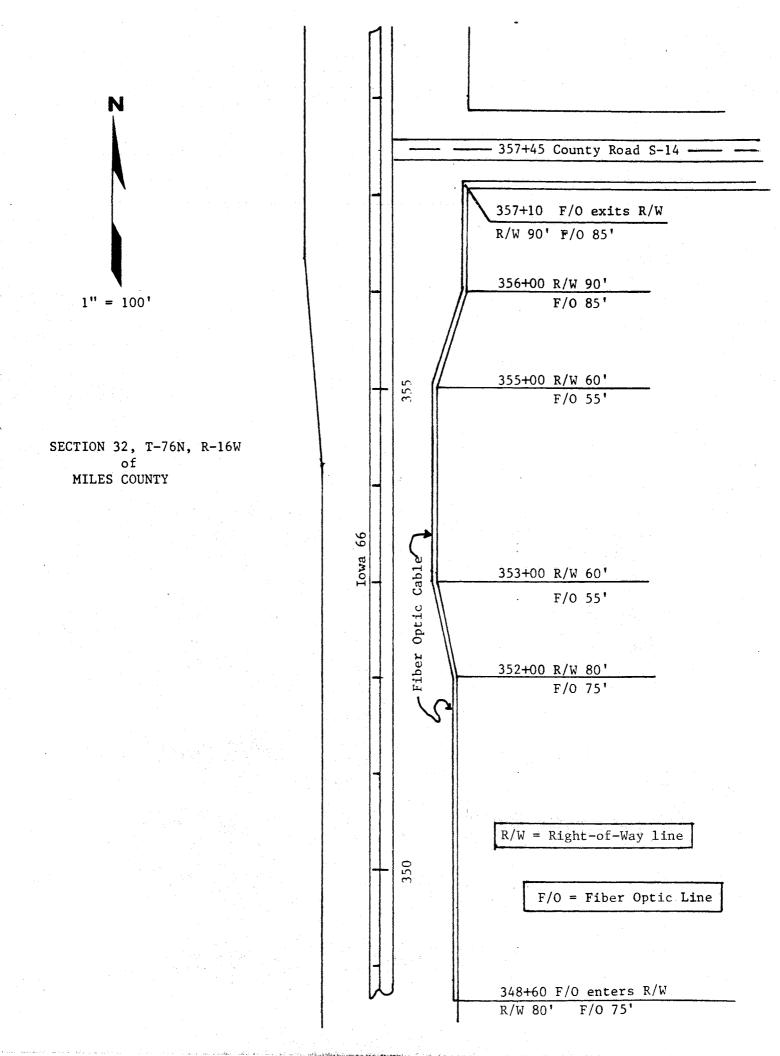
Utilities to be located as near the highway right of way line as physically possible.
