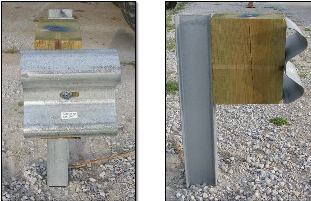
Figure 114. Test Setup to Measure Guardrail Bolt Torque
