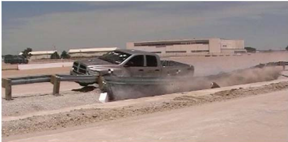
Figure 33. Sequentials – Test No. LSC-2 and LS-DYNA Simulation with Silverado-v2
