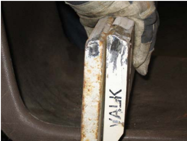
Photo 1: Conventional (L) & Underbody Blades
