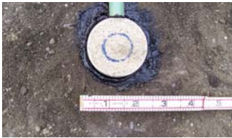
Soil Pressure Cell Installation Method 1
