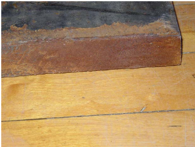
Figure 7. Test Blade With Carbide Completely Worn Off
