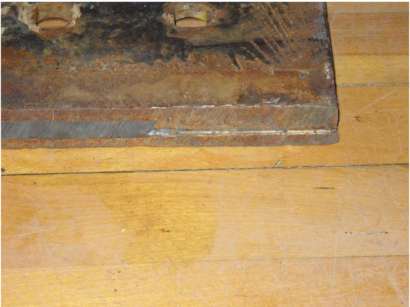
Figure 9. Control Blade with Carbide Gone Near the leading Edge
