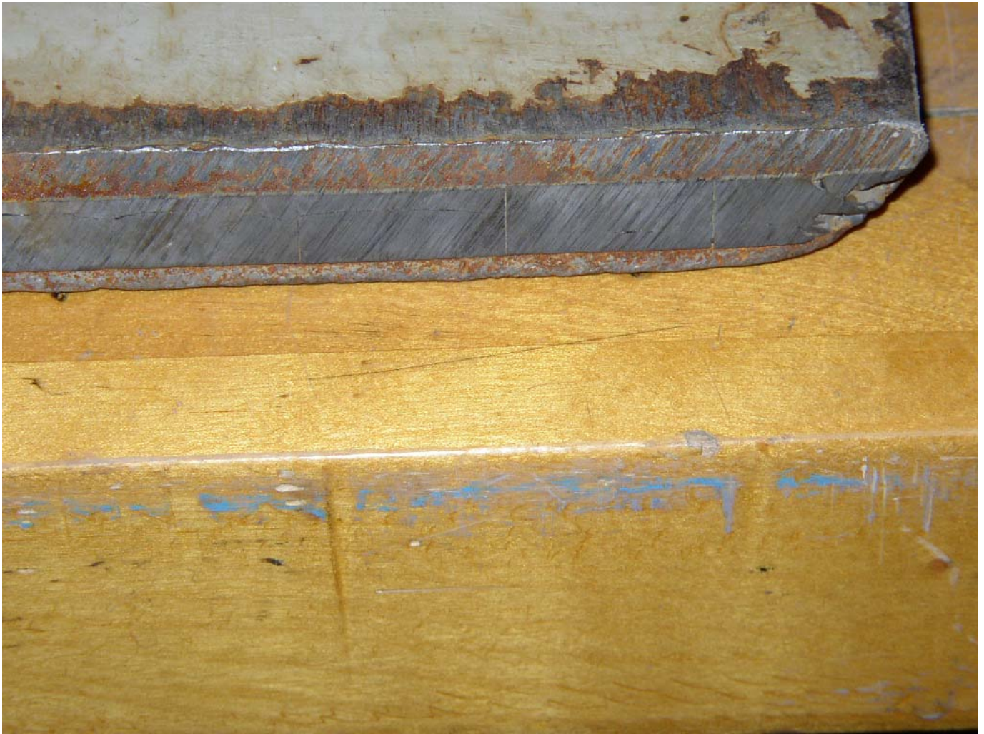
Figure 10. Control Blades With Some Carbide Remaining
