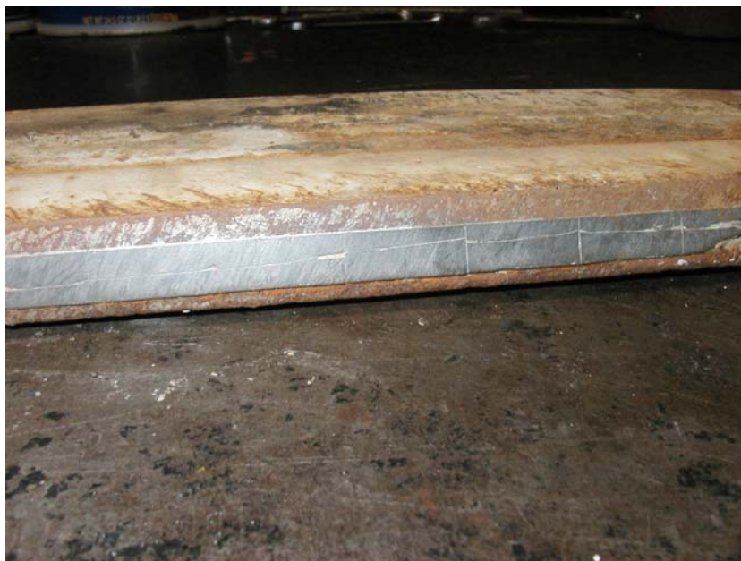
Figure 1a. Hairline Cracks Spreading to Adjacent Carbide Inserts
