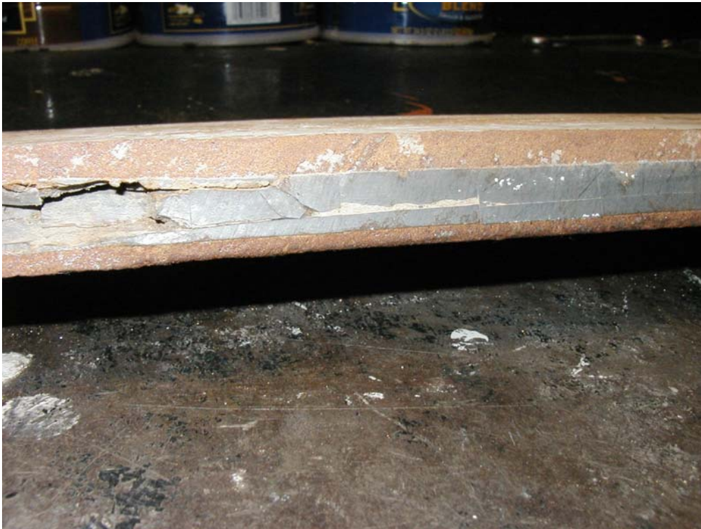
Figure 1b.Edge View Where Carbide has Broken
