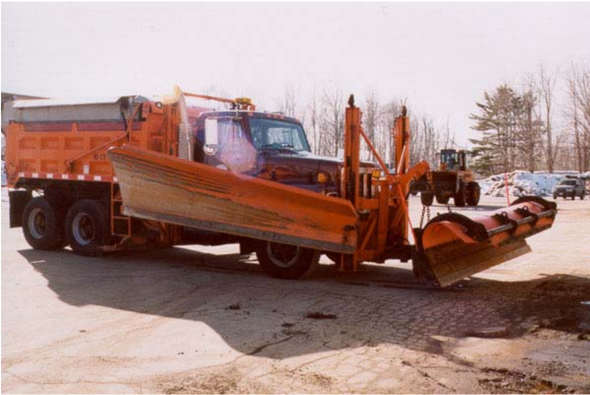
Figure 2. Truck Outfitted with Test Blades on Both Front and Wing Plows
