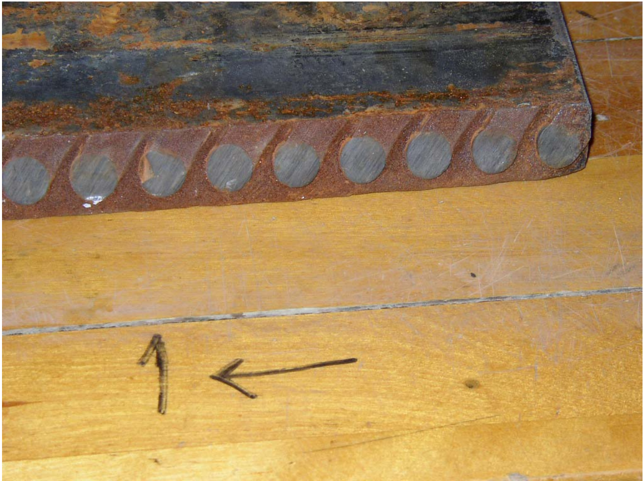
Figure 6. Close-up of Carbide Inserts. Photo shows the right side of the left-most blade (as viewed from “driver’s” side of plow.)
