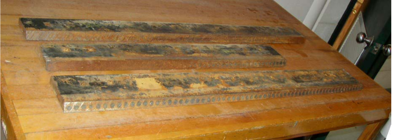
Figure 5. Test Blades after Removal, Showing Remaining Round Carbide Inserts
