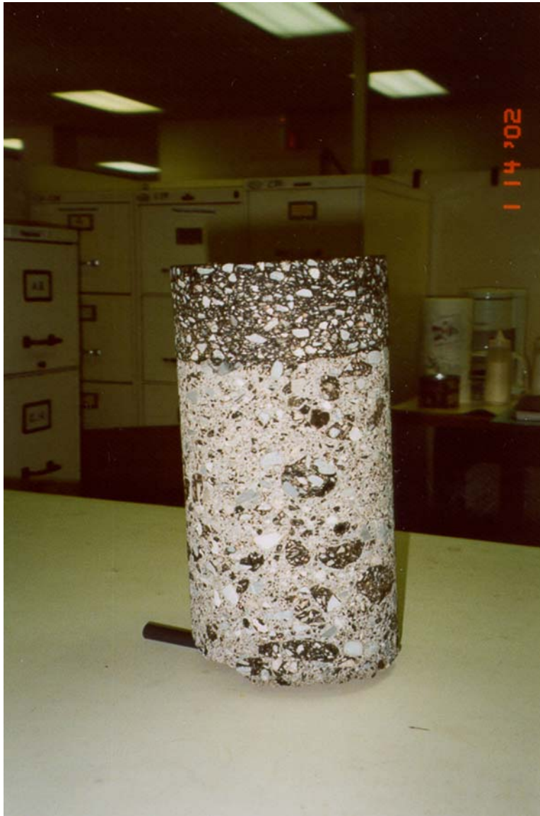
Figure 25. Core Showing PC-RAP & HMA Asphalt Surface Pavement
