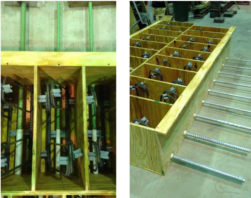
Figure 3-2. Wooden forms with epoxy-coated (left) and galvanized (right) test bars
