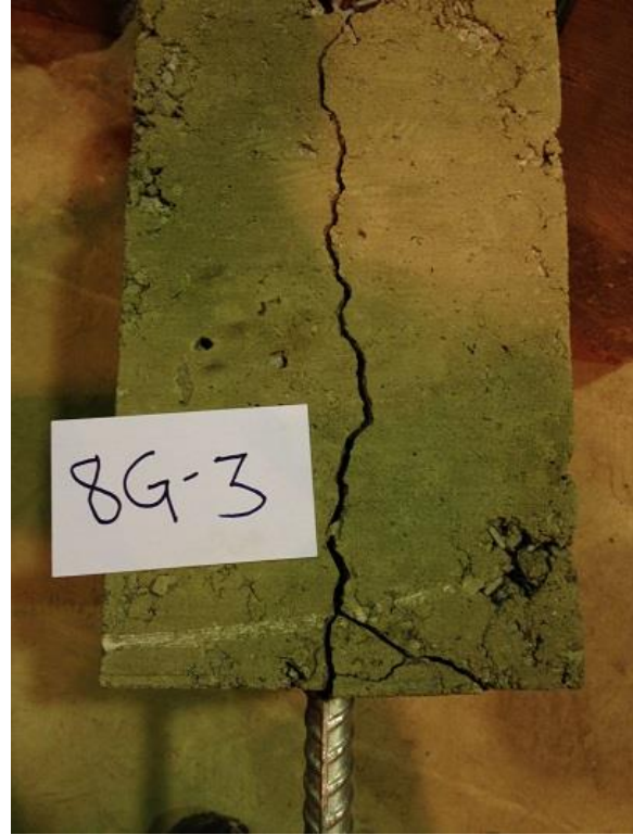
(b) Specimen with #8 galvanized test bar
