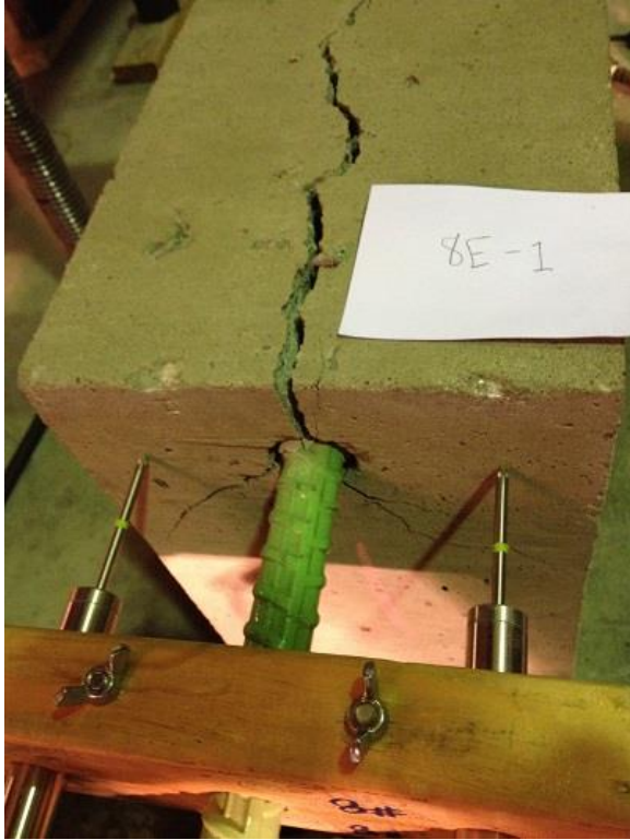
(a) Specimen with #8 epoxy-coated test bar
