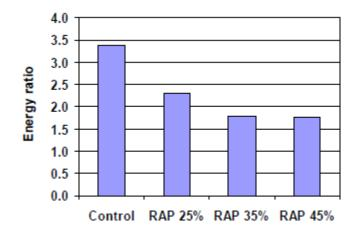
**Figure 11:** Energy ratio results for varying RAP mixes (Kim et al. 2007)
