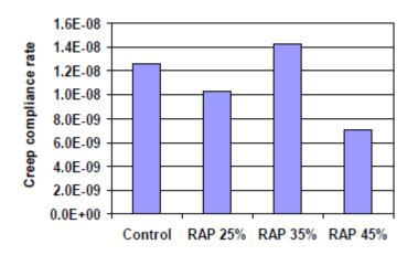
Figure 9: Creep compliance rate for varying RAP mixes
