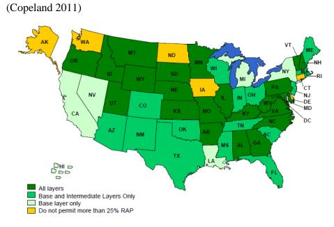
**Figure 2:** States that permit more than 25% RAP in HMA pavement (Copeland 2011)
