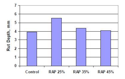
**Figure 5:** APA test result for varying RAP mixes
