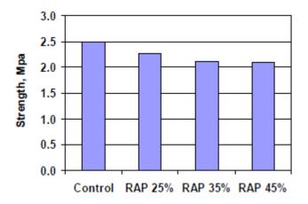
**Figure 7:** Tensile strength test results for varying RAP mixes (Kim et al. 2007)
