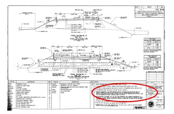
"5. CONSTRUCT EMBANKMENT TO DESIRED SUBGRADE SURFACE ELEVATION USING ITEM 203.03. ONCE THE DESIRED SUBGRADE ELEVATION HAS BEEN REACHED. PLACE 1.5 MINIMUM SURCHARGE (ITEM 203.03). OBSERVE A TWO MONTH WAITING PERIOD. THIS WAITING PERIOD MAY BE REDUCED BASED ON RESULTS FROM FIELD INSTRUMENTATION. REMOVE SURCHARGE UNDER ITEM 203.03
