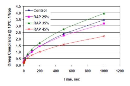
**Figure 10:** Creep compliance rate for varying RAP mixes (Kim et al. 2007)
