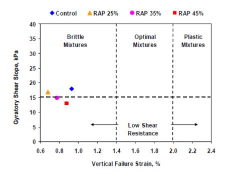
**Figure 6:** Servopac gyratory shear test results for varying RAP mixes (Kim et al. 2007)
