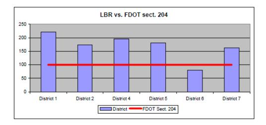
Figure 15: Average RCA limerock bearing ratio
