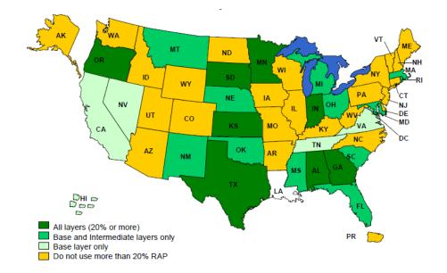
**Figure 3:** States with more than 20% RAP usage in HMA pavement (Copeland 2011)
