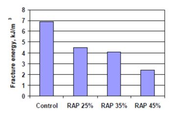
**Figure 8:** Fracture energy results for varying RAP mixes (Kim et al. 2007)
