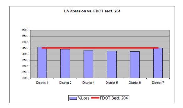
Figure 16: Average RCA LA abrasion loss compared to FDOT Specifications 204 for natural aggregates
