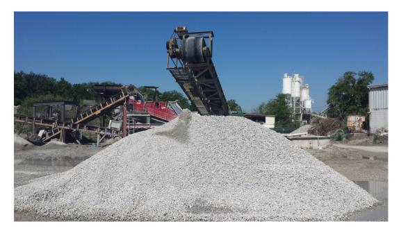
Figure 23: Crushed concrete at Florida Concrete Recycling facility in Gainesville, FL
