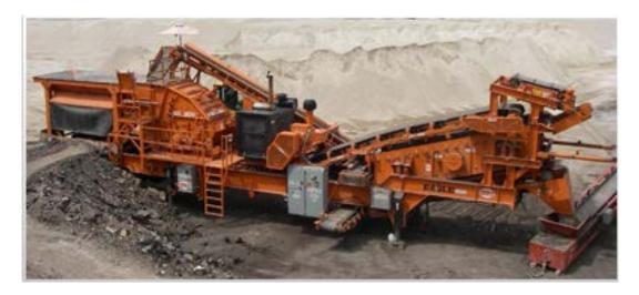
Figure 18: Crush-It portable concrete crusher
