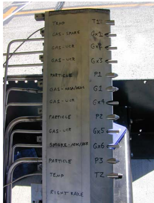
Figure 6a: Starboard sampling probe stand (left). Figure 6b: Probe rake with different probes (right)
