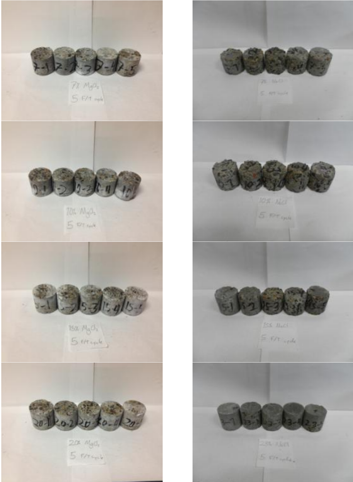
Figure 3.13: Lab concrete samples exposed to 5 F/T cycles in MgCl_2 and NaCl solutions, respectively
