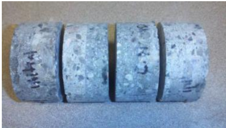
Figure 7.5: Samples of cement based overlays including overlay (0.5'') and concrete (0.5'') used for gas permeability test
