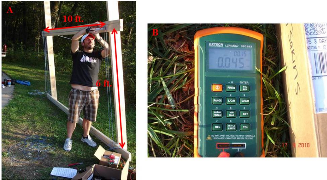
Figure 11. Construction of the custom-made antenna. (A) the 10 x 6 ft. 2 2-wire loop custom RFID antenna developed by Papanicolaou research team; and (B) The LCR meter used to measure the custom RFID antenna inductance, L (45 \mu\text{H} ).
