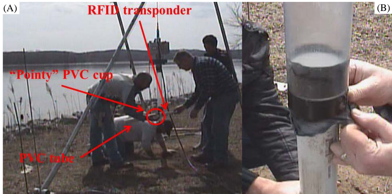
Figure 19. Using the vibracore. (A) The transponder is placed into a PVC core tube and secured with a “pointy” PVC cup. (B) The PVC joint is wrapped up with electrical tape to increase friction between the acrylic and the PVC tubes. Once the desired depth is reached, the vibracore is pulled up, while the RFID transponders have been buried into the stream bed.
