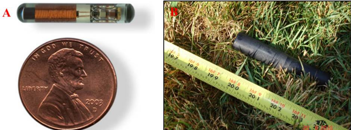
Figure 4. RFID transponders. (A) 23-mm glass encased transponder, with a penny for a size comparison; and (B) 120-mm long transponder. Both transponders are from Texas Instruments.
