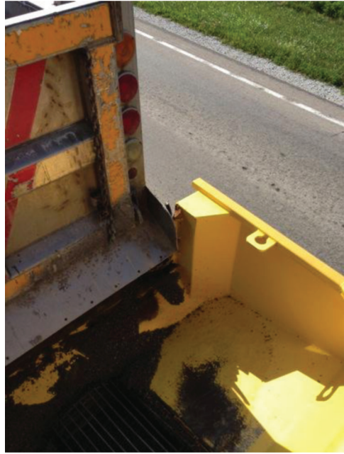
Figure 4.8 Damage to the chipper box.
