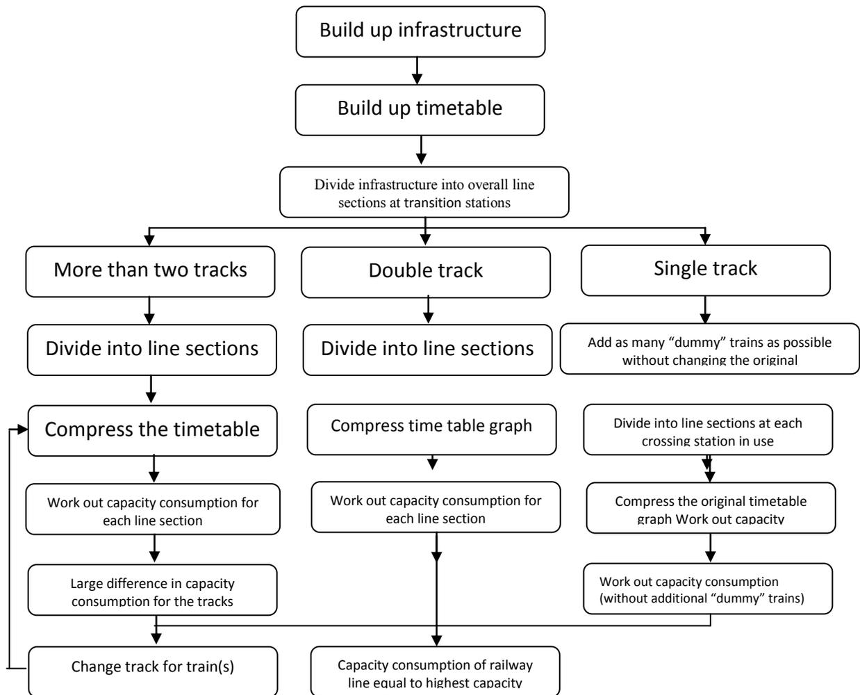
Figure 6: Workflow of measuring capacity consumption of railway lines [29].
