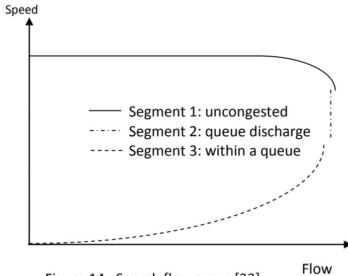
Figure 14. Speed-flow curve [33]
