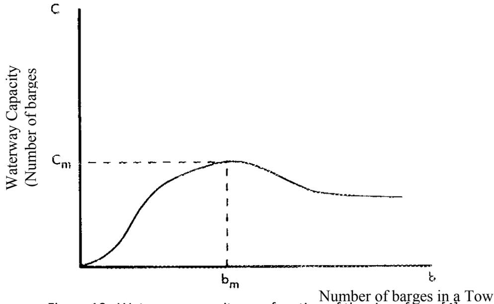
Figure 10. Waterway capacity as a function of the size of tow [4]
