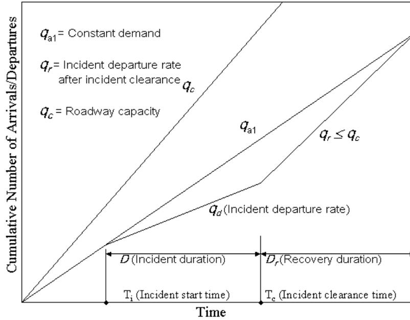
Figure 16. Incident Delay Diagram - Deterministic Model (one arrival rate) [42]
