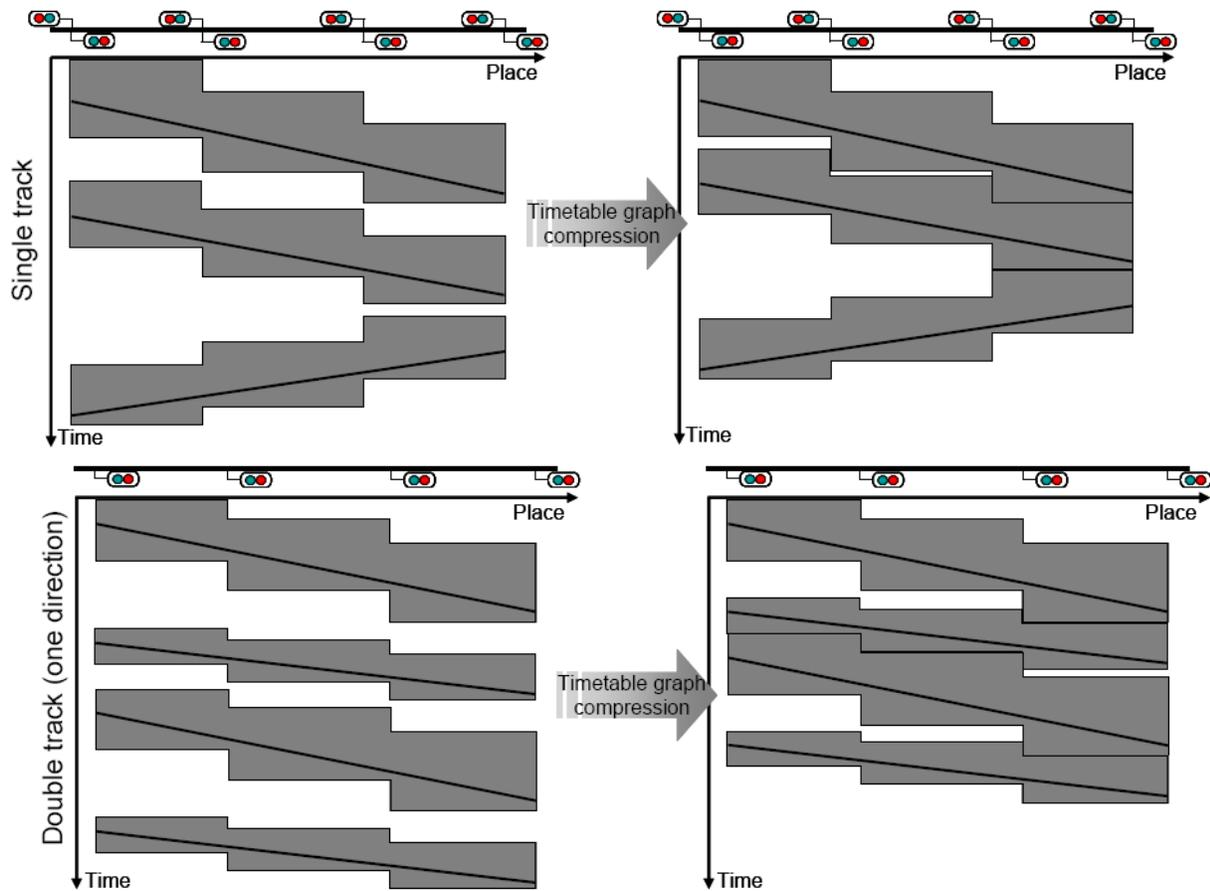
Figure 3. Compression of timetable graph according to the UIC406 capacity method. Partly based on [23]
