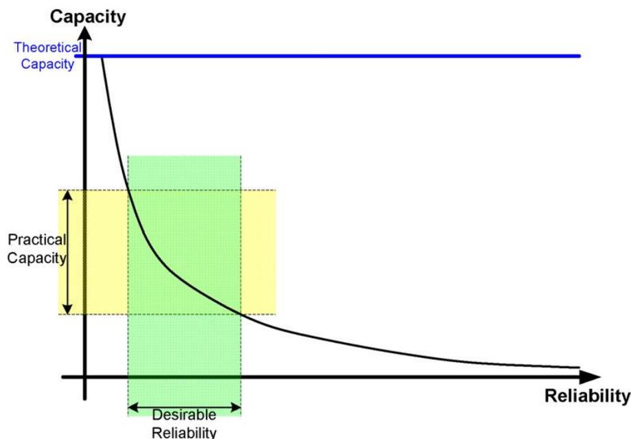
Figure 1. Practical capacity involves the desirable reliability level [12].
