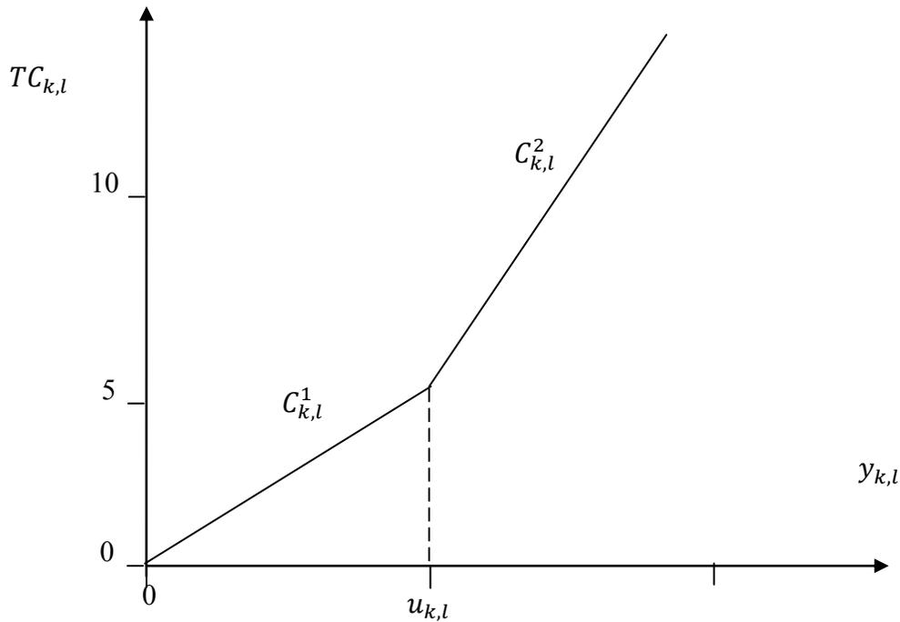
Figure 28. Piecewise linear approximation of the cost-flow function
