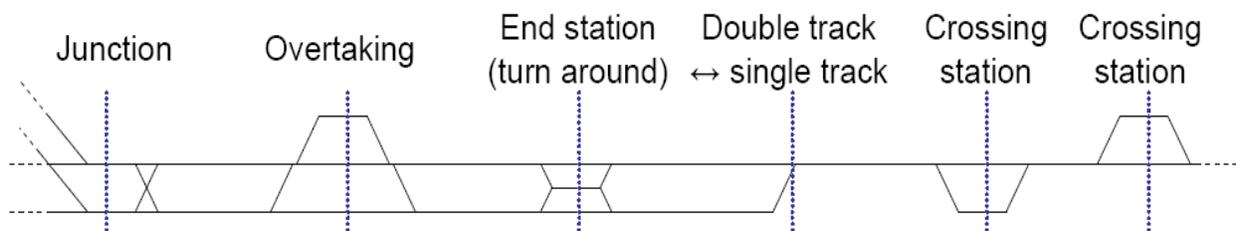
Figure 4. Division of railway line into line sections [24, 25]
