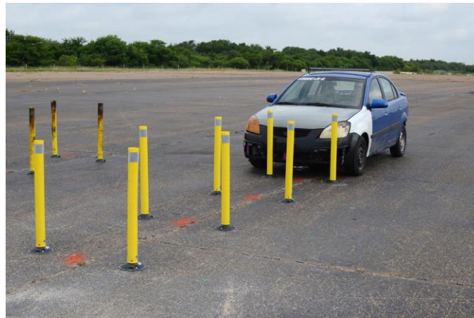
Figure 1. MASH 1100C Modified Test Vehicle for Evaluation of Delineators.
