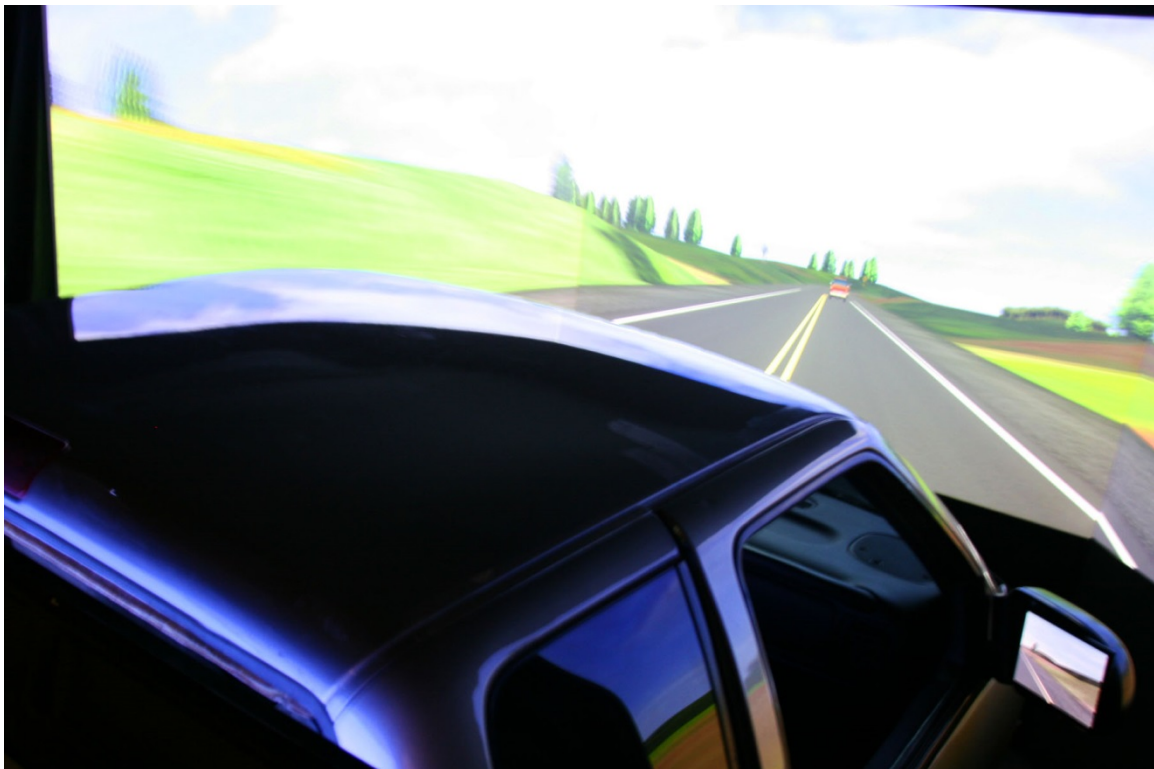
Figure 12. Overhead view of Chevy S-10 cab with the 3 Main forward displays and right-side mirror display visible. The instrument cluster, left side mirror, and center rear view mirror are not visible.
