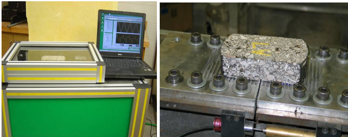
Figure 2. Overlay Tester Equipment and Sample.
