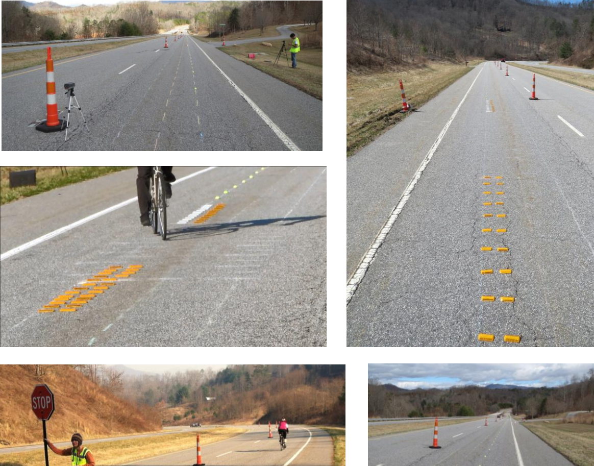
FIGURE 7 Clockwise from top left: looking east down course showing radar gun and video camera placement; looking west uphill showing first gap subjects approach as they ride through the course; looking east down the course showing tennis ball line between scenario A and B stations; at top of course looking east showing ITRE researcher signaling to NCDOT traffic controllers upstream; close-up of subject crossing a gap while bicycling at high speed.
