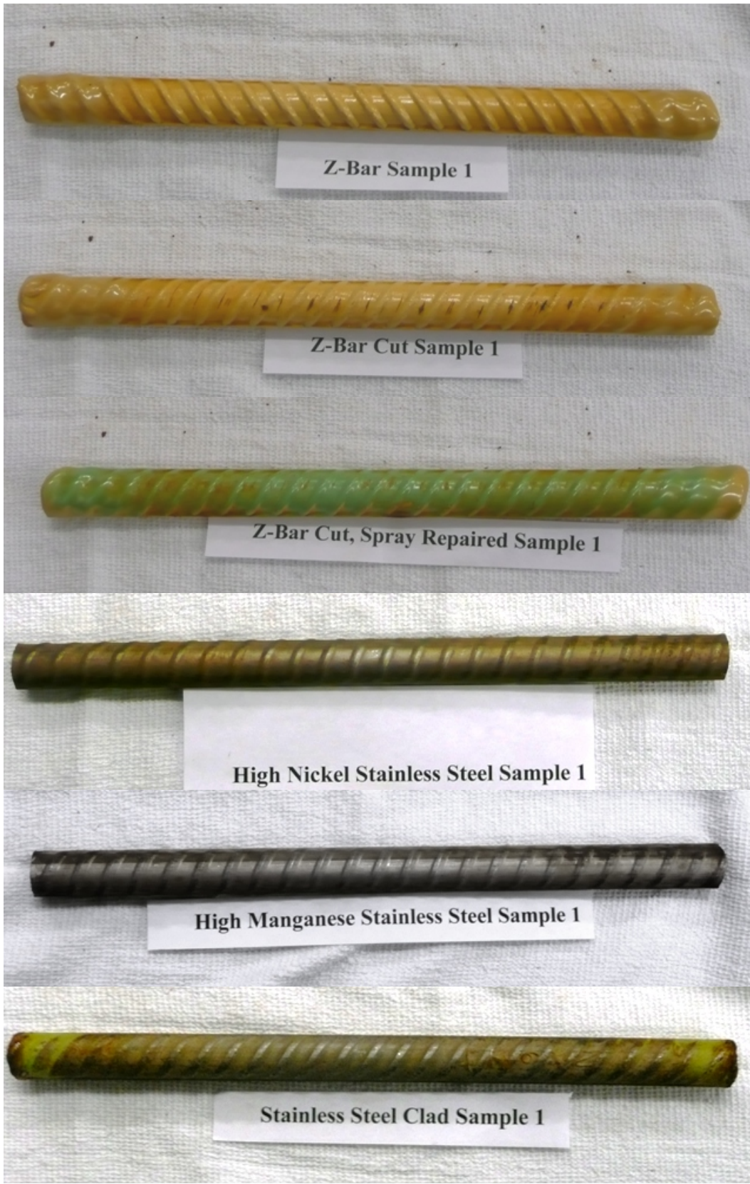
Figure 1 (cont.) Images of each bar in series 1 in their final condition following 260 salt water immersion cycles.
