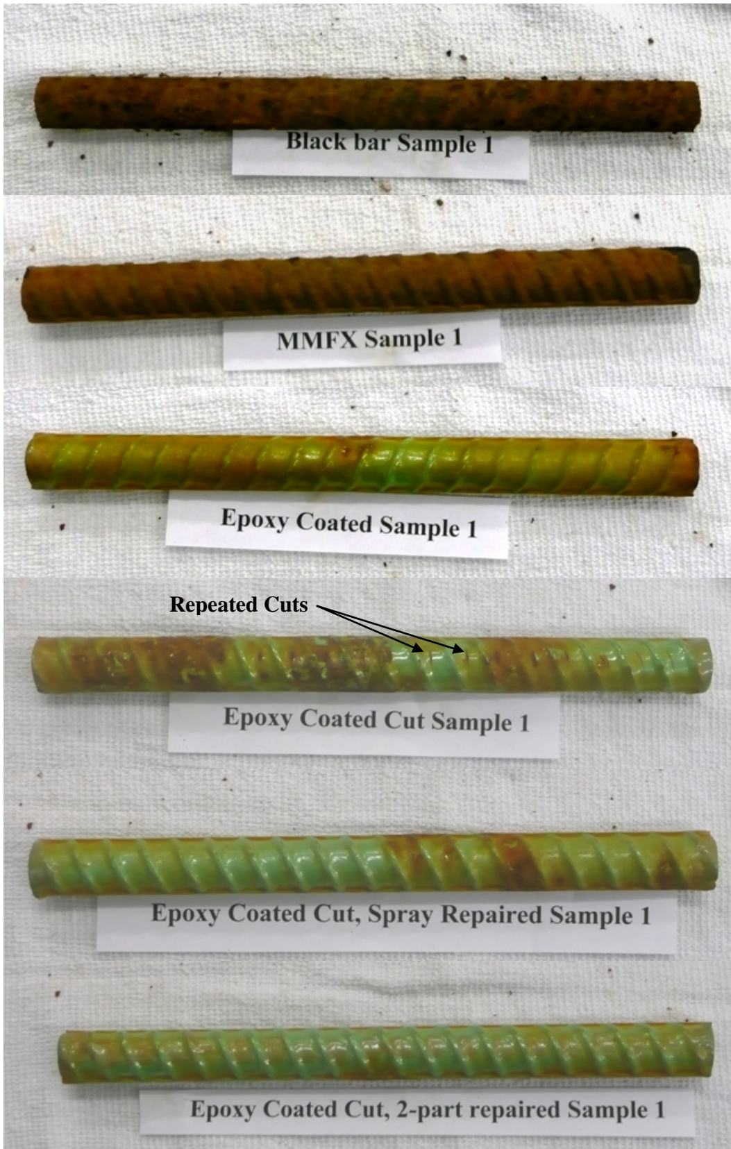
Figure 1. Images of each bar in series 1 in their final condition following 260 salt water immersion cycles.
