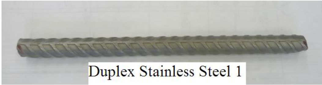
Figure 1 (cont.) Images of each bar in series 1 in their final condition following 260 salt-water immersion cycles.
