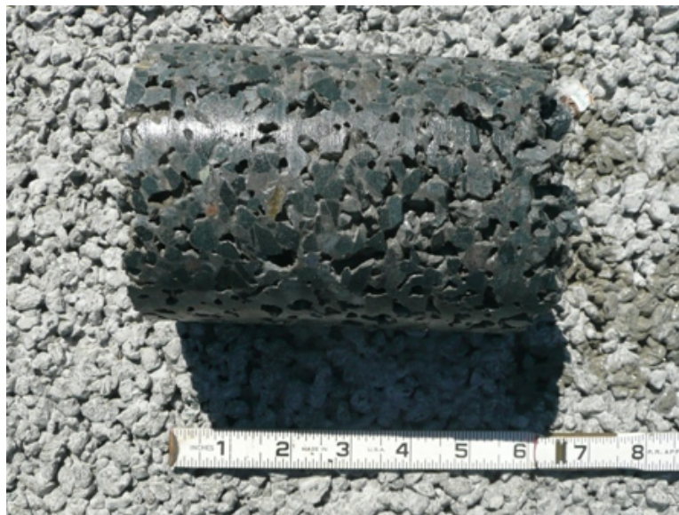
Figure 5. Core 1, taken from a visually and audibly sound portion of the lot.
