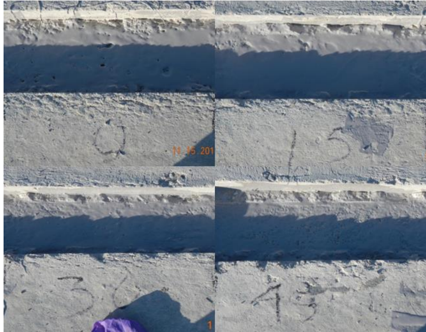
Figure 0.13 0, 15, 30, and 45 minutes after epoxy bonding agent application
