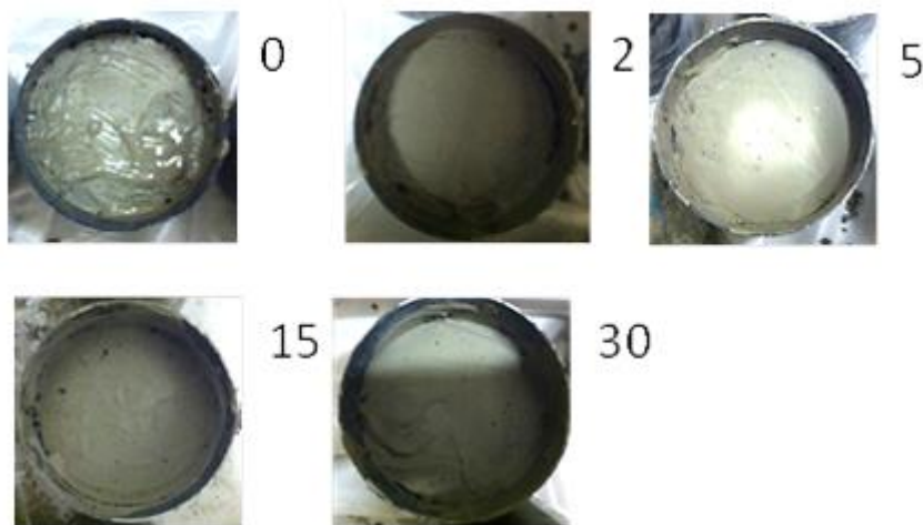
Figure 0.5 Waiting time effects for 0.5 W/C grout
