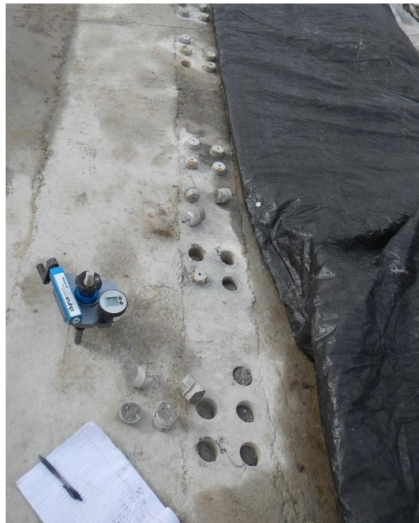
Figure 0.17 Pull-off tensile testing
