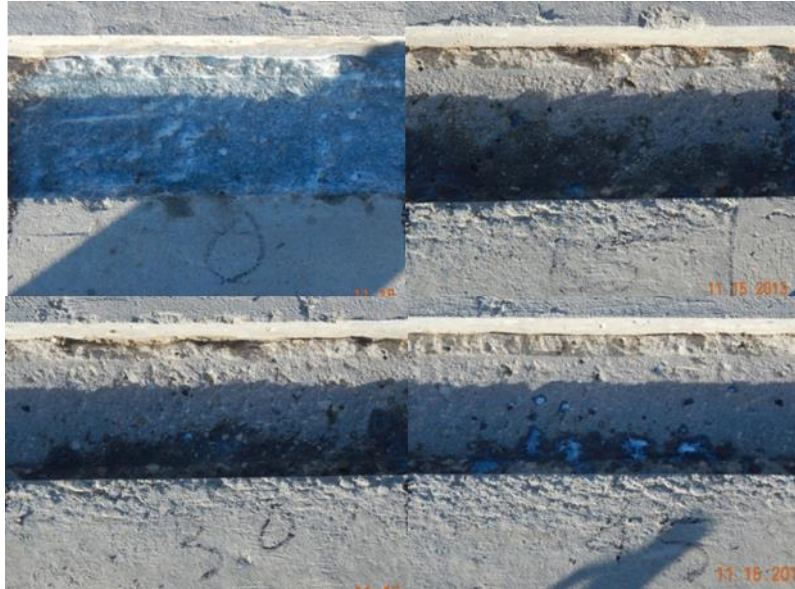
Figure 0.15 0, 15, 30, and 45 minutes after acrylic bonding agent application
