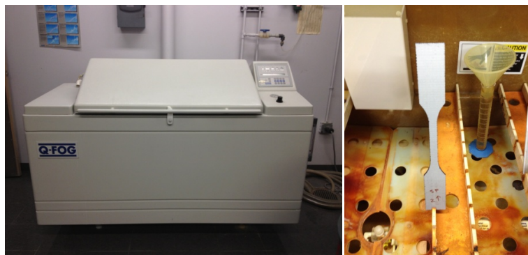
Figure 7-3 Slat Fog Apparatus (Left image) GFRP Specimen Exposed to Salt Fog (Right image)
