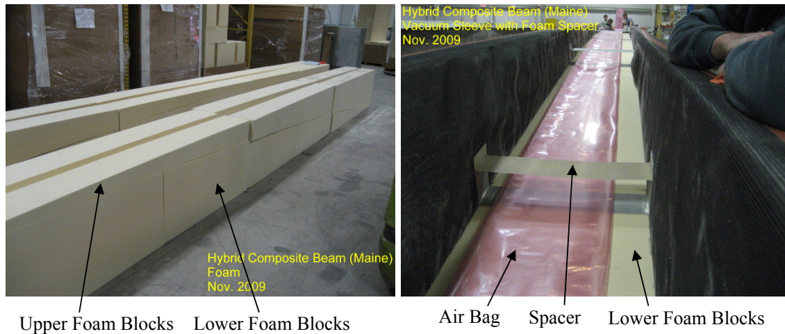
Figure 2-5 Cut and Preparation of the foam blocks (left image) Placement of the air bag and Spacers (right image)
