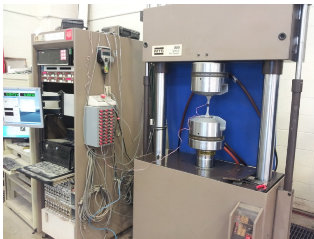
Figure 7-6 Tensile Coupon Test for FRP Specimen via MTS880 Universal Testing Machine
