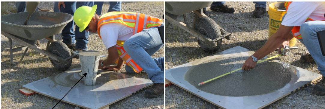
Figure 4-8 The Slump Flow Test Without J-ring
