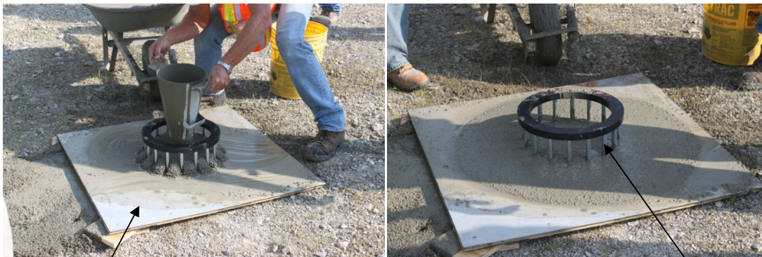
Figure 4-9 The Slump Flow Test With J-ring
