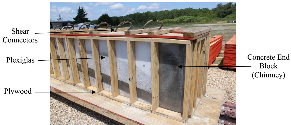
Figure 4-7 Mock-Up Beam (one day after pour)
