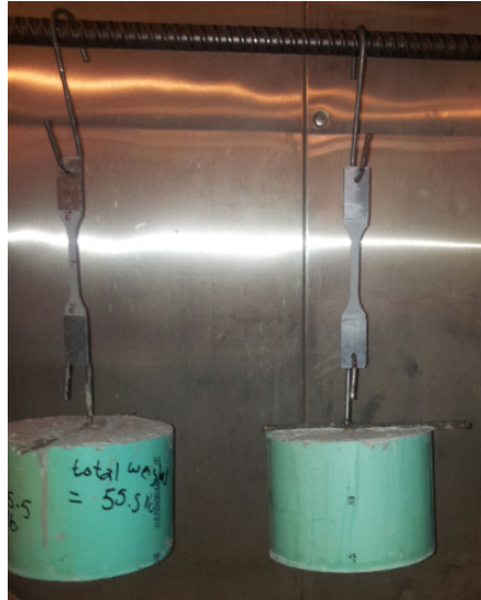
Figure 7-5 FRP Specimens Subjected to Sustained Stress and Thermal Cycles in the Environmental Chamber
