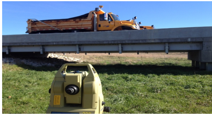
Figure 5-12 Two MoDOT Truck Simulating Load Cases on B0478
