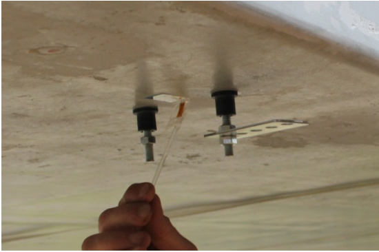
Figure 3-16 FRP Strain Gauge Placement, M-Bond Adhesive
