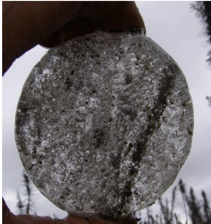
Figure 9. Appearance of wedge ice, sample obtained by SIPRE corer (9-Mile Hill area, Dalton Highway, Alaska)
