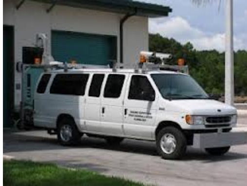
Figure 1: Specialized Van for IRI Data Collection
