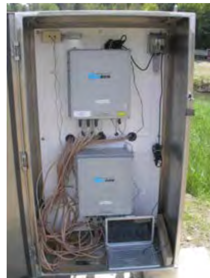
Figure 3-22: Data Acquisition System (Loggers) near Approach Slab
