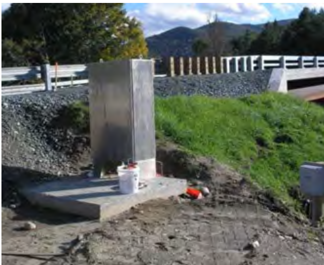
Figure 3-22: Data Acquisition System (Loggers) near Approach Slab
