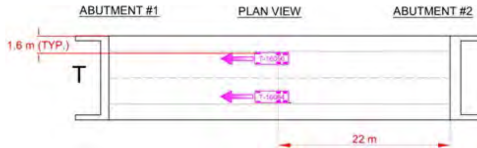
Figure 5-8: Middlesex Load Testing Truck Locations (Transverse Arrangement)
