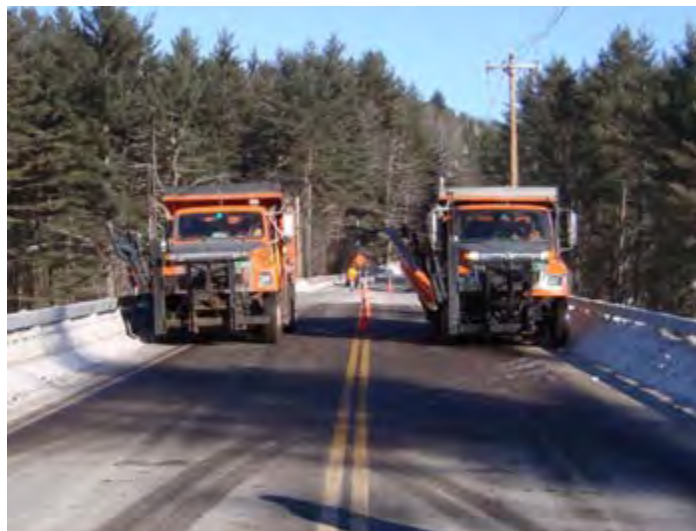
Figure 5-4: Middlesex Load Testing (Transverse Arrangement of Trucks)
