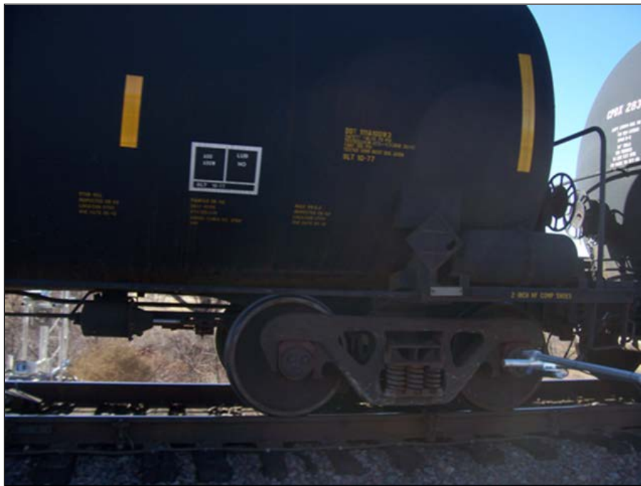
Figure 1. Braking Tank Car with Proper Piston Travel
