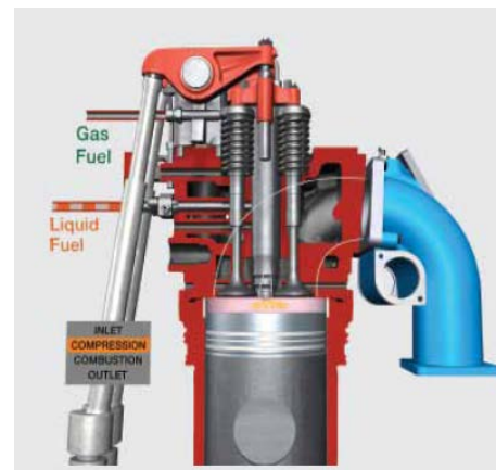
Figure 2(i). Diesel/Gas Dual Fuel Engine Cylinder Cutaway
