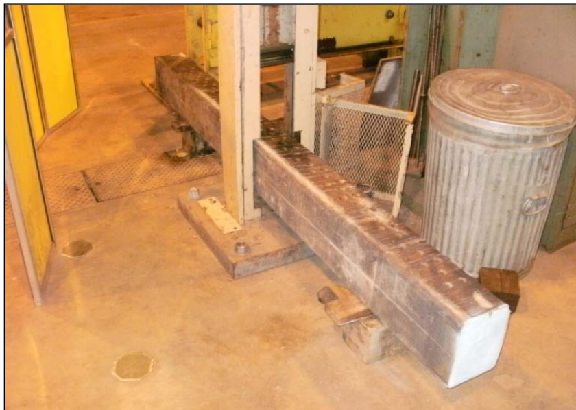
Figure 30. Drop fixture with tie placed on its side. Note the supports are still spaced at 60 inches apart, simulating the loading of other AREMA tests.
