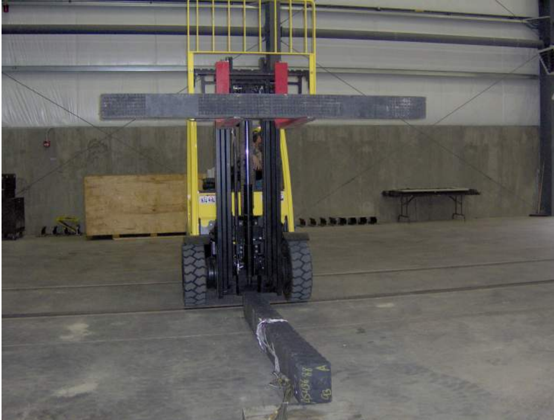
Figure 11. Configuration 3: (Photograph) Full load about to be dropped on an instrumented plastic composite tie.
