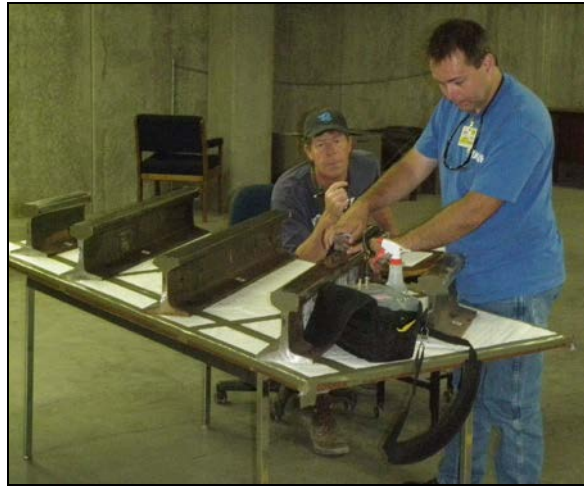
Figure 11. Inspection Participant Using Conventional Ultrasonic Testing Equipment
