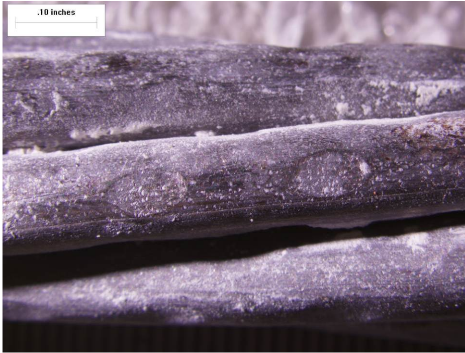
Figure 4.1. Example of elliptical deformations on seven-wire strands from a pre-2003 tie.
