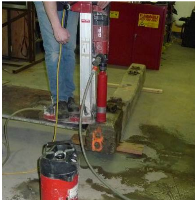
Figure 4.4. SGH retrieving a full-depth vertical core sample from a tie.
