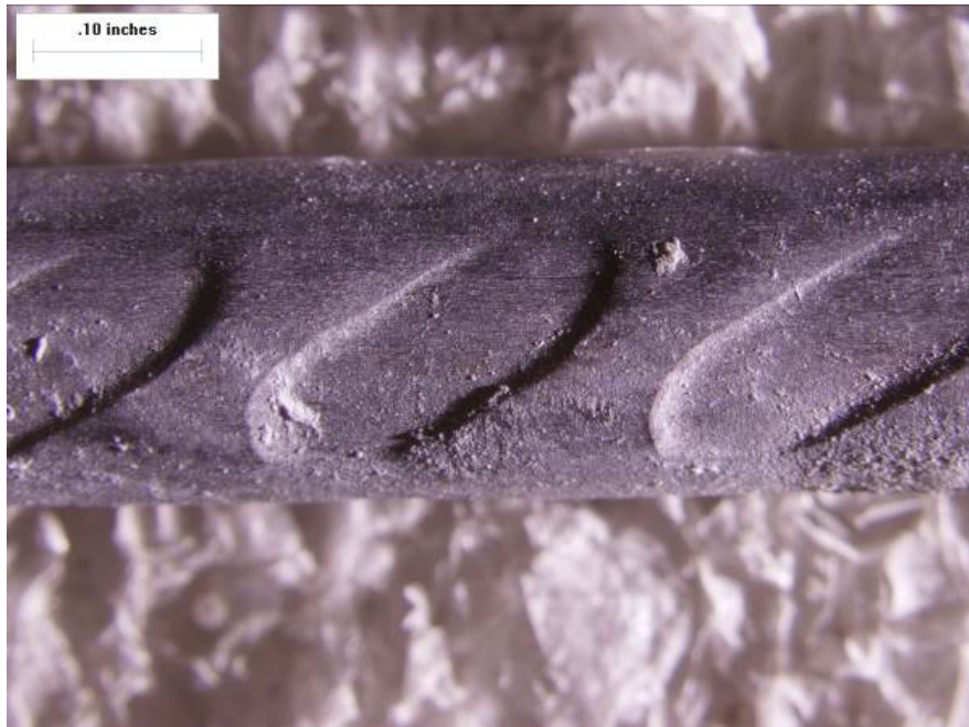
Figure 4.2. Example of elongated elliptical deformations on a single-wire strand from a post-2003 tie.
