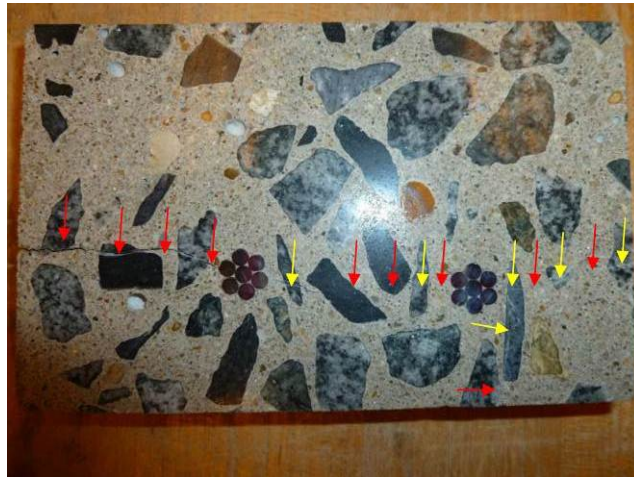
Figure 4.17. Crack condition on the polished section from Core C17-3. Red arrows point to direction and extent of cracks; yellow arrows point to the reactive aggregates.
