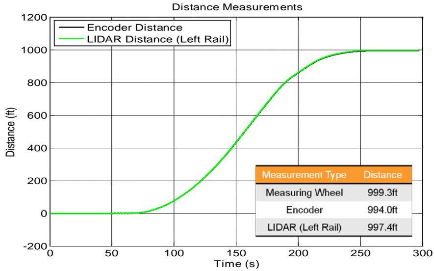
Figure 29: The encoder vs. LIDAR distance measurements based on scaling during calibration from Run #1 (Calibration Run #2)
