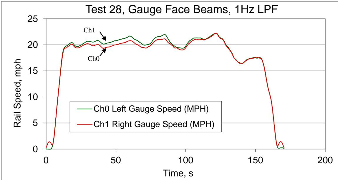
Figure 11: A comparison of filtered, LIDAR speed from right and left rail vs. time of a Hy-Rail test
