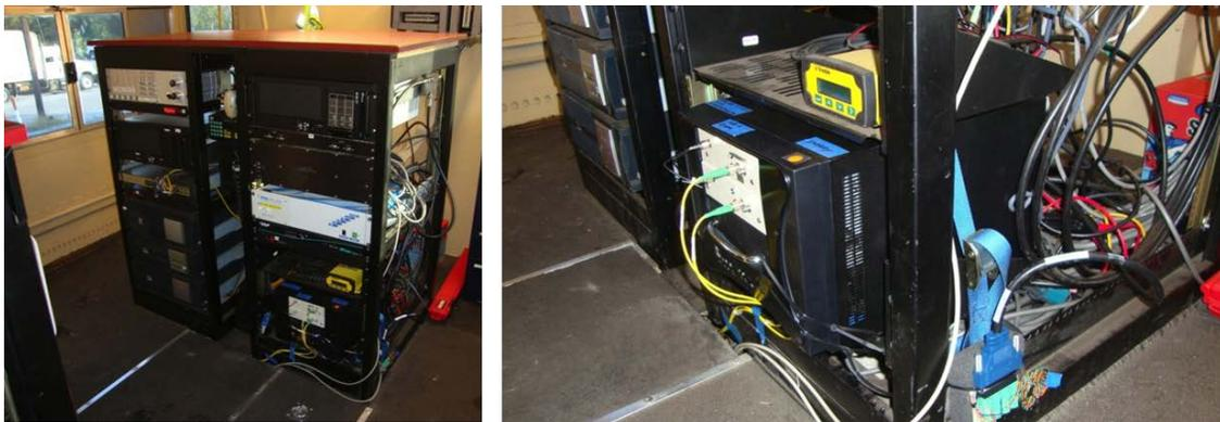
Figure 23: LIDAR computer installed onboard the track geometry car and linked to KVM system
