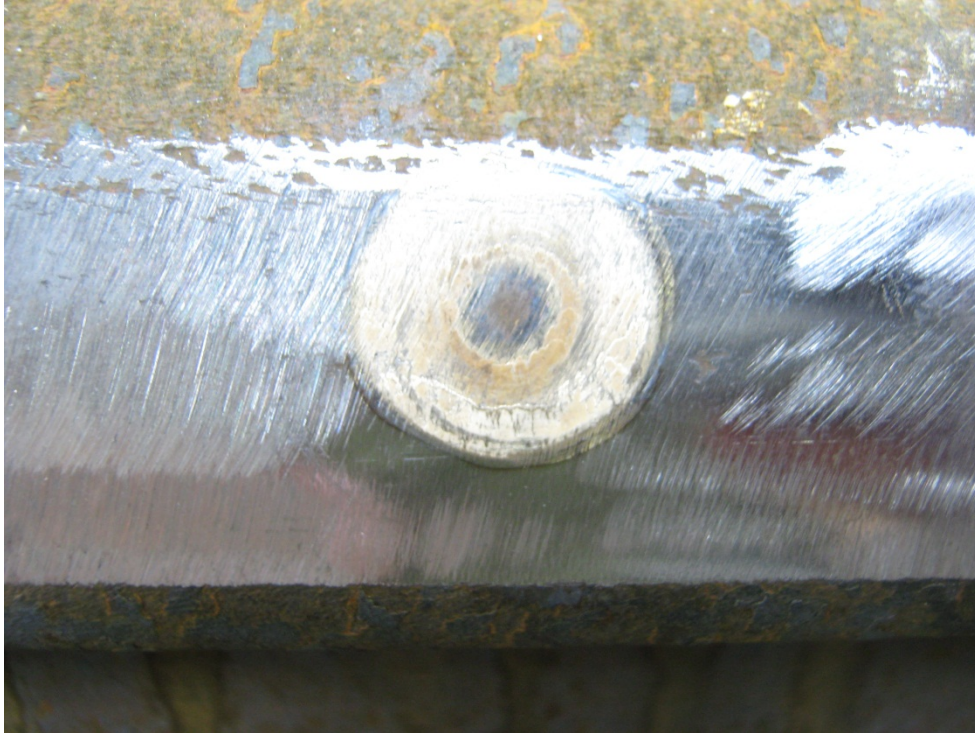
Figure 52. IFW Shear Test Failure Surface
