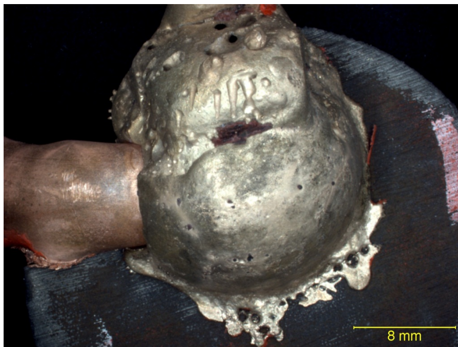
Figure 1. Exothermic RWI Joint
