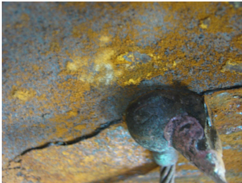
Figure 43. CAD Weld after Corrosion Test
