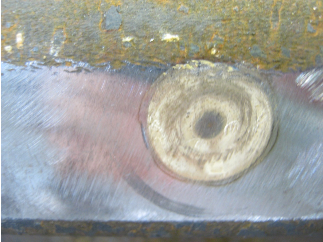
Figure 76. IFW Joint Displaying Characteristics of Axial Misalignment
