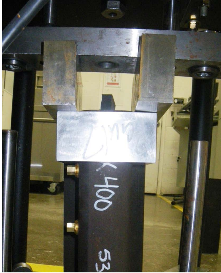
Figure 53. Impact Fixture Applied to IFW Joint
