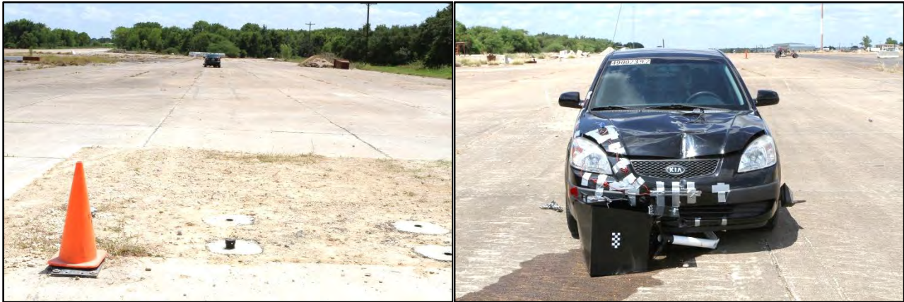
Figure 4.13. Vehicle/Installation Positions after Test No. 490023-9-2.
