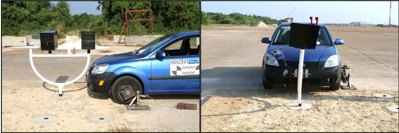
Figure 5.4. Vehicle/Installation Geometrics for Test No. 490023-9-3.
