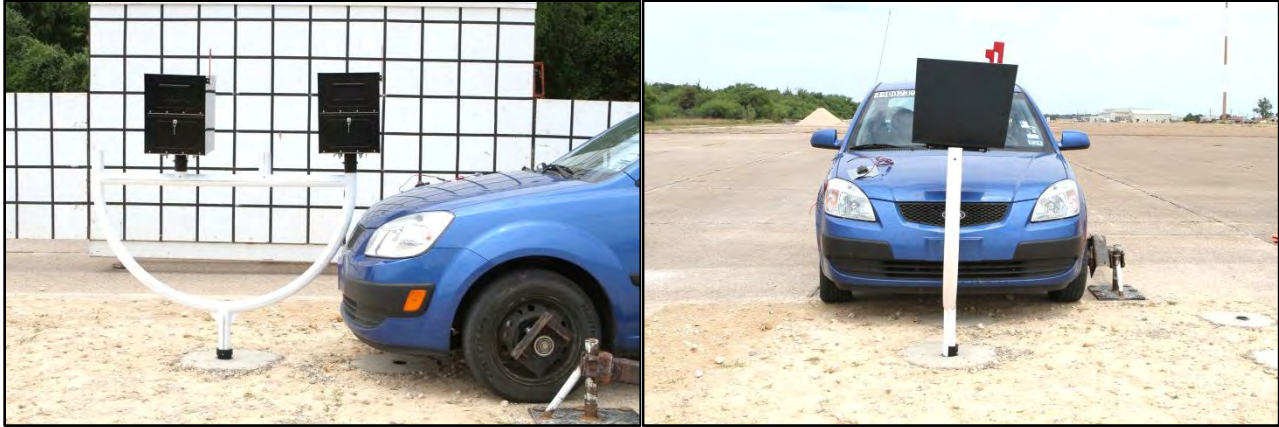
Figure 5.11. Vehicle/Installation Geometrics for Test No. 490023-9-4.
