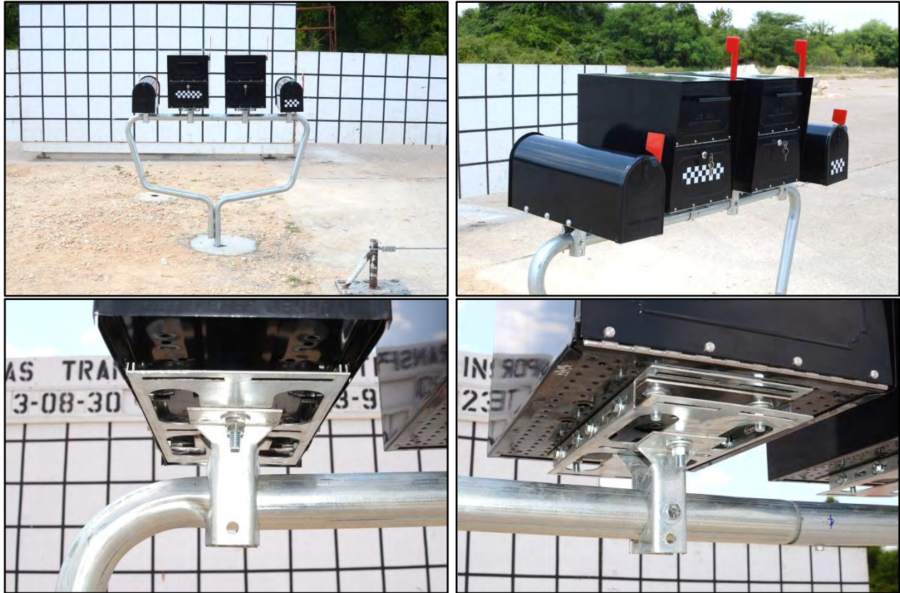
Figure 6.17. Locking Architectural Mailboxes and Standard Mailboxes before Crash Test No. 490023-9-6.
