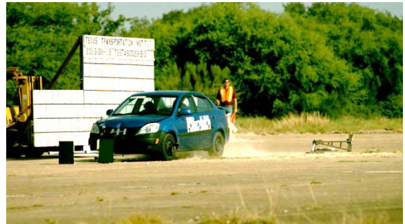
Figure C1. Sequential Photographs for Test No. 490023-9-3 (Perpendicular and Oblique Views) (Continued).
