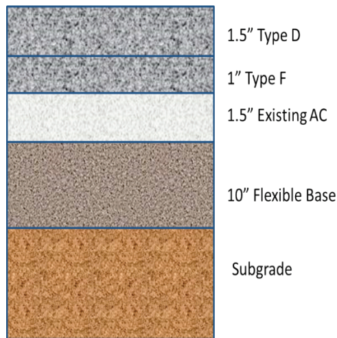
Figure 1. Pavement Structure of SH 15 Test Sections.
