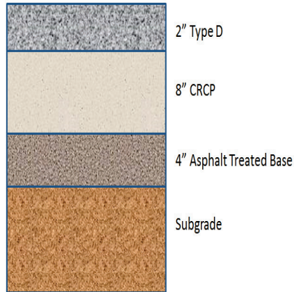
Figure 3. Pavement Structure of Loop 820 Test Sections.
