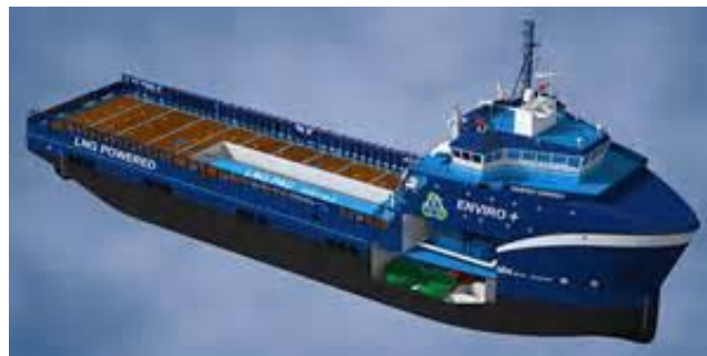
Figure 15 LNG powered offshore supply vessel
