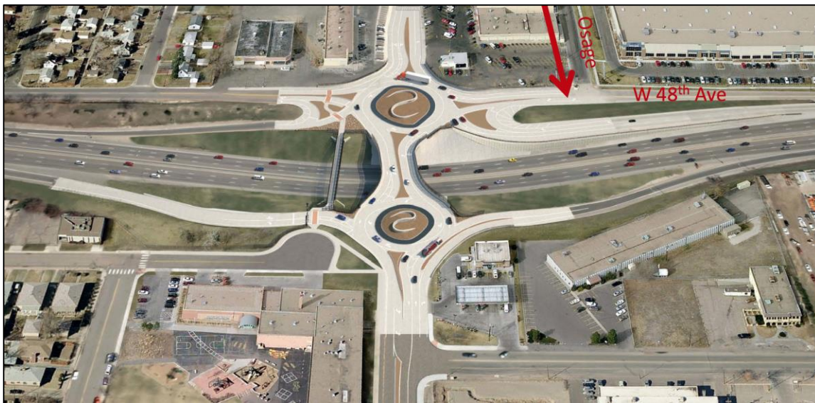
Figure 4.3 BIM Model graphic showing converging streets and the need for the roundabouts
