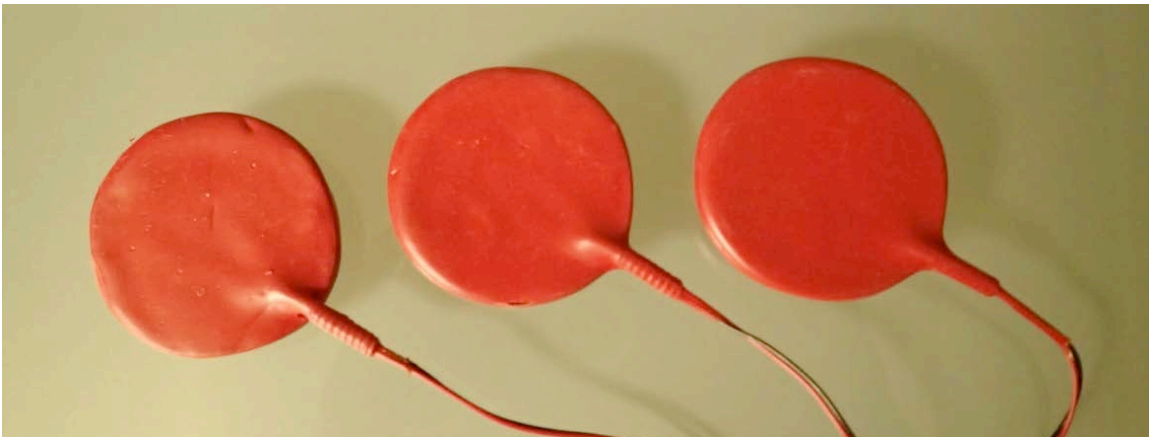
Figure 17: Photograph of the new eStress TM gauge system. The future replacement of strain gauges.
