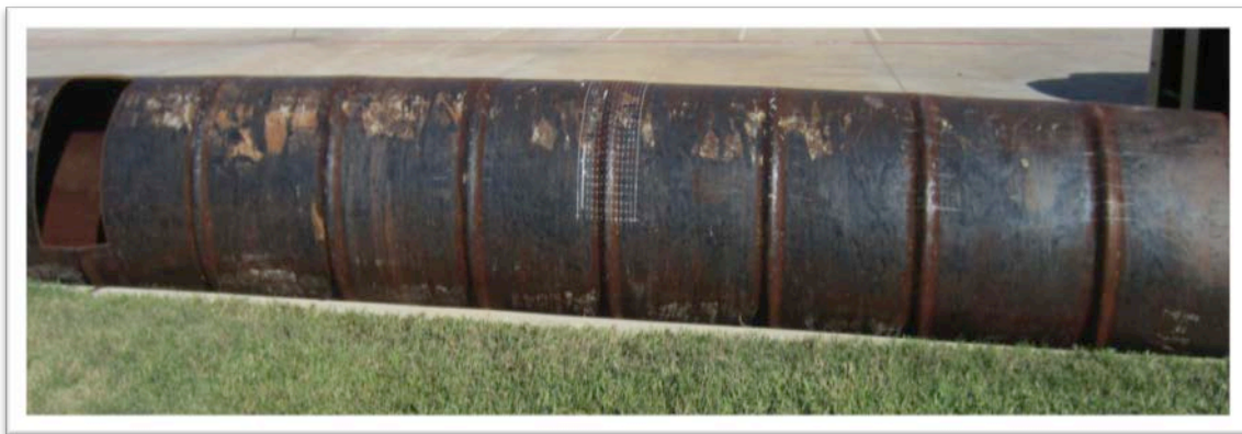
Figure 1: Section of steel pipeline with wrinkle bends to be analyzed for residual stress levels.
