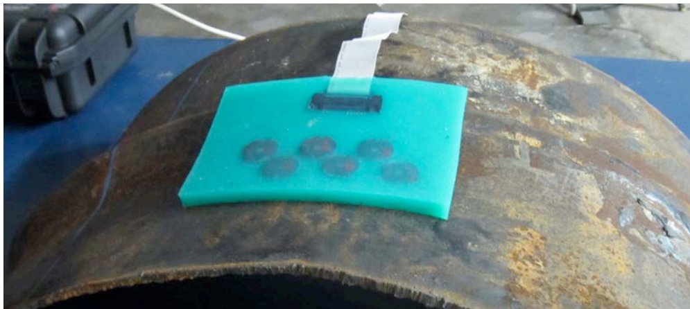
Figure 7: Photograph of the first prototype of the floppy mat system for damaged pipelines.
