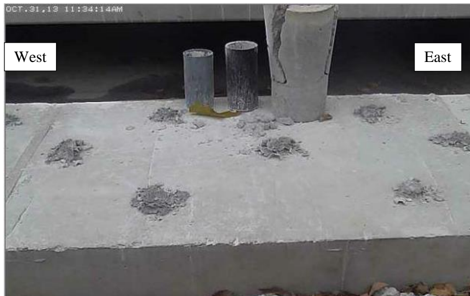
Figure 23. Chemical splitting on day six (after 144 hours)
