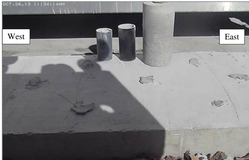
Figure 18. Chemical splitting on day one (after 24 hours)
