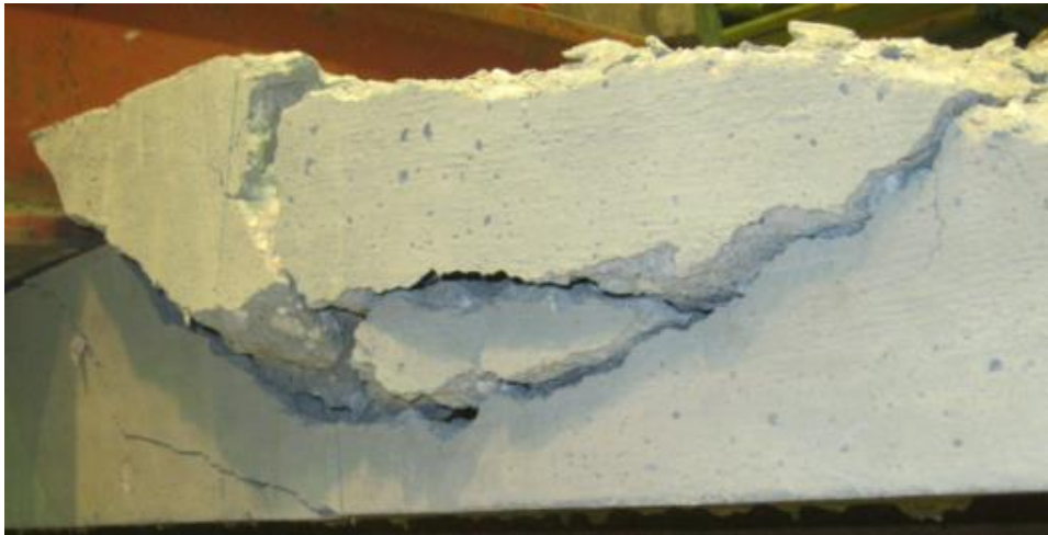
Figure 32. Fifth peeling test (3 shear studs) (Dang 2013)
