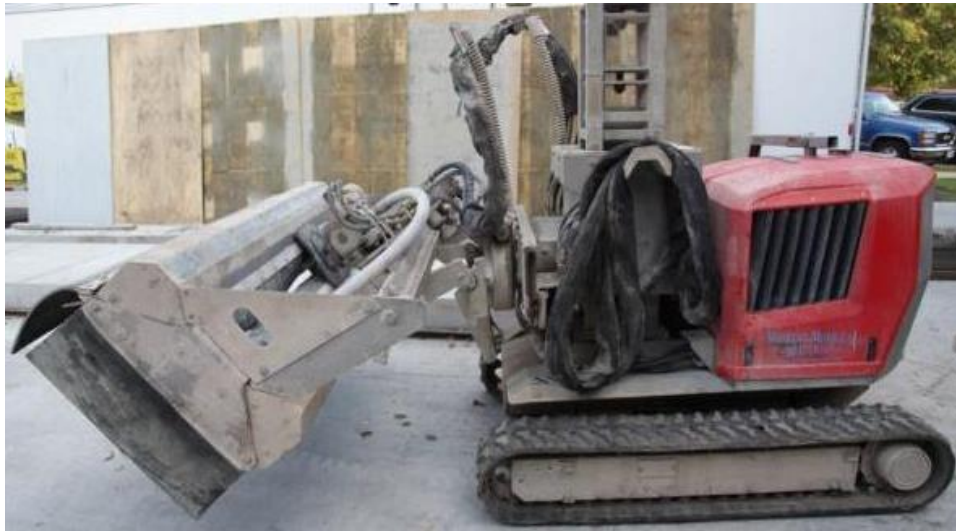
Figure 4. Demolition unit (Dang 2013)
