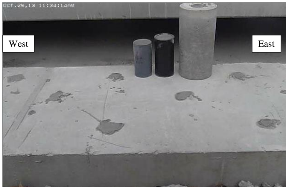
Figure 17. Chemical splitting specimen and the grout
