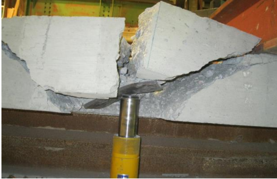
Figure 29. Second peeling test (3 shear studs) (Dang 2013)
