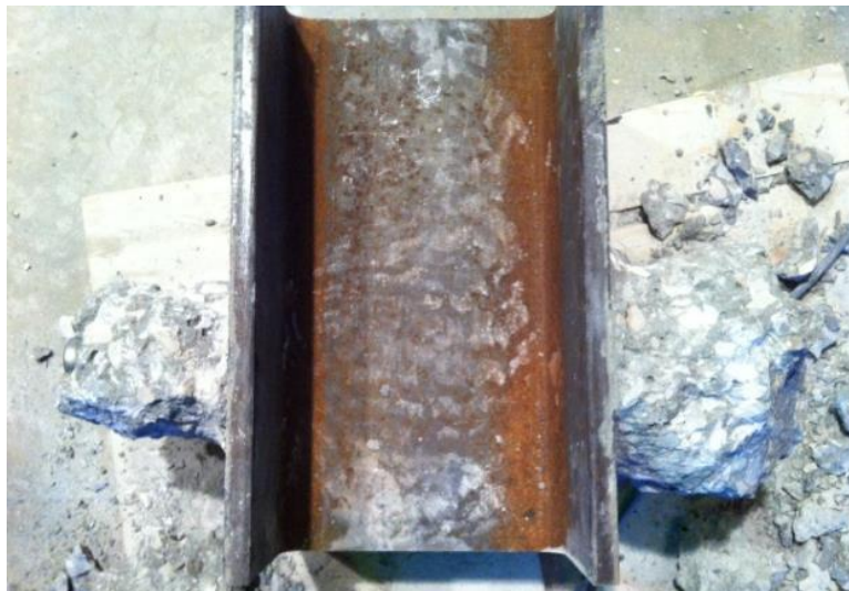
Figure 40. Partially removed concrete specimen (Dang 2013)
