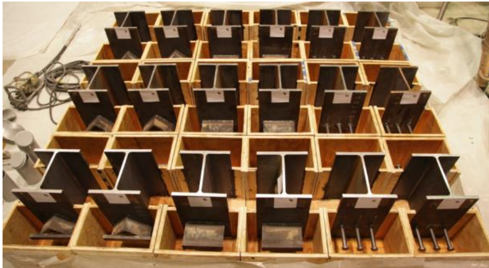
Figure 38. Constructed steel specimens and concrete formwork (Dang 2013)
