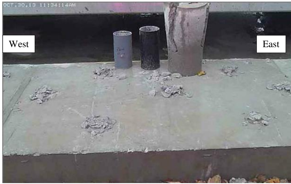
Figure 22. Chemical splitting on day five (after 120 hours)
