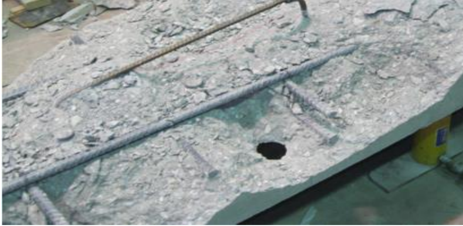
Figure 31. Fourth peeling test (3 shear studs) (Dang 2013)
