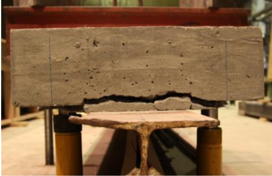
Figure 27. Front view of the first peeling test (3 shear studs) (Dang 2013)
