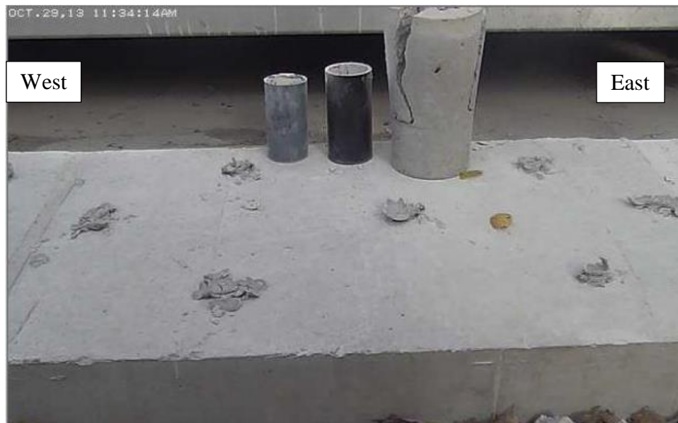
Figure 21. Chemical splitting on day four (after 96 hours)
