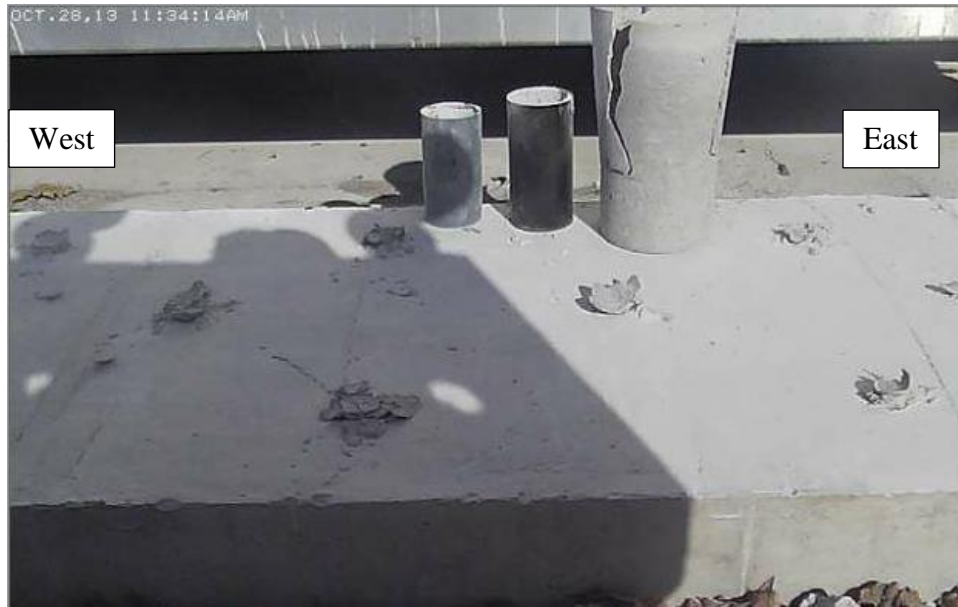
Figure 20. Chemical splitting on day three (after 72 hours)
