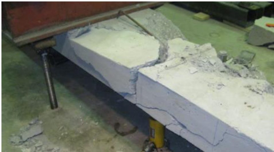
Figure 30. Third peeling test (3 shear studs) (Dang 2013)
