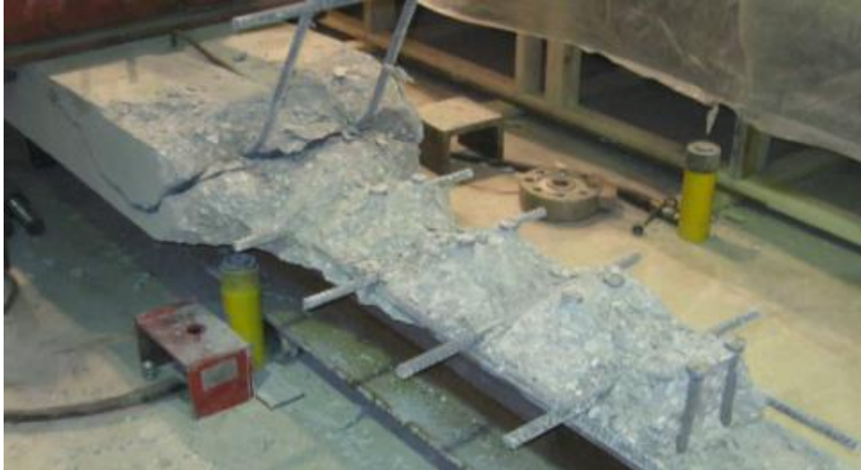
Figure 35. Second peeling test (2 shear studs) (Dahlberg 2014)
