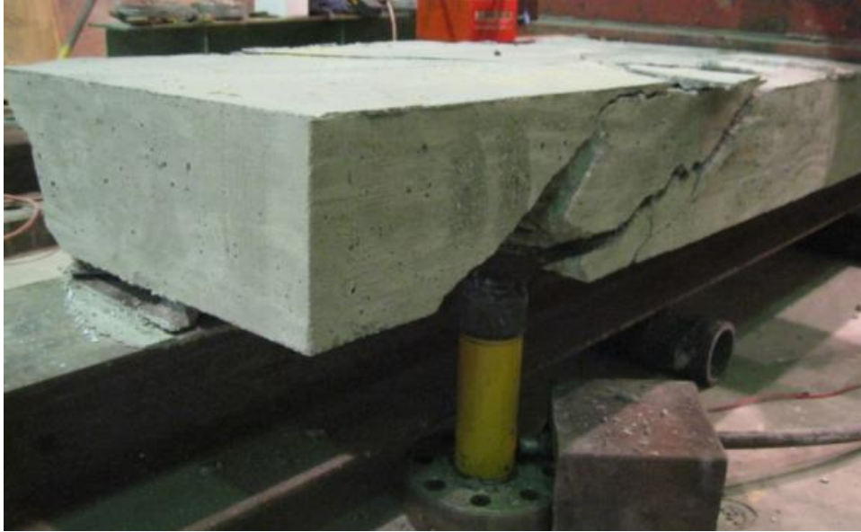
Figure 33. Side view of the first peeling test (2 shear studs) (Dahlberg 2014)
