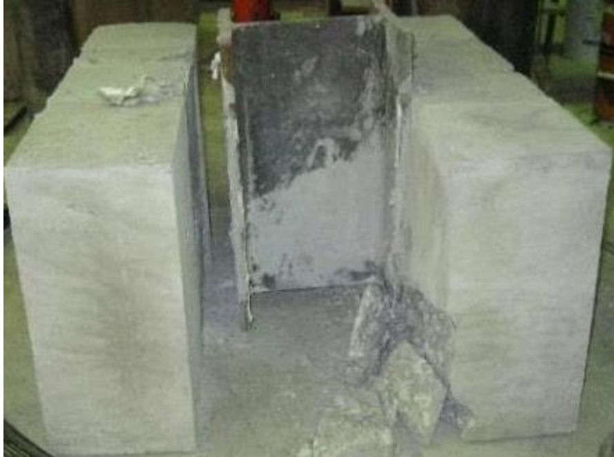
Figure 45. Typical shear connector failure (Dang 2013)
