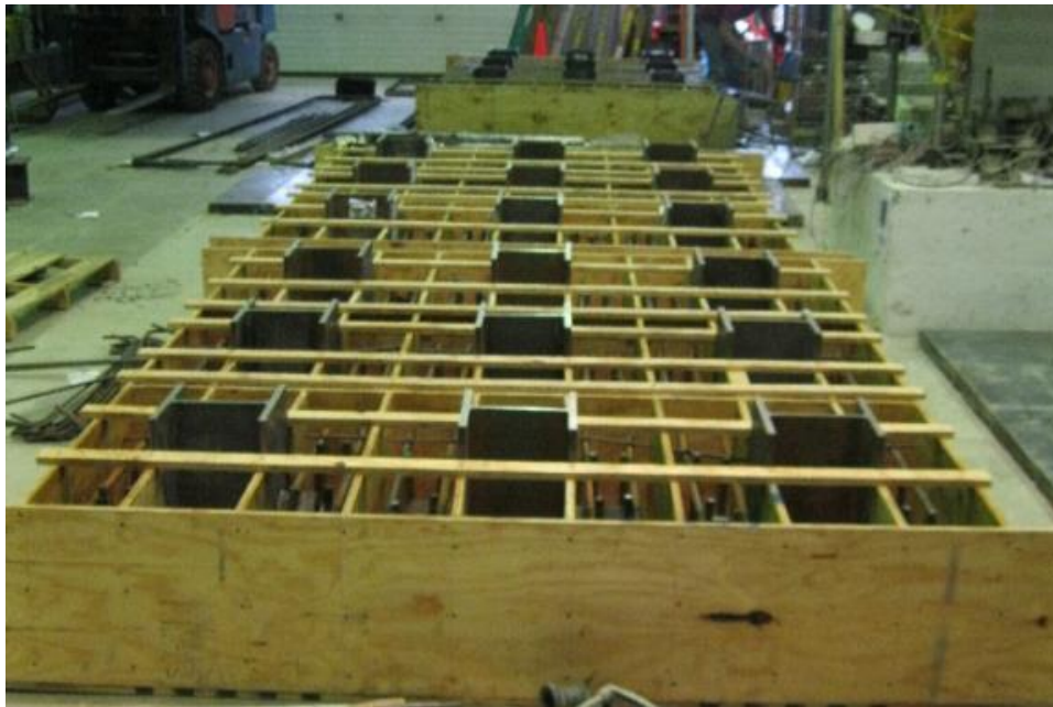
Figure 42. Partially removed concrete specimens and formwork (Dang 2013)
