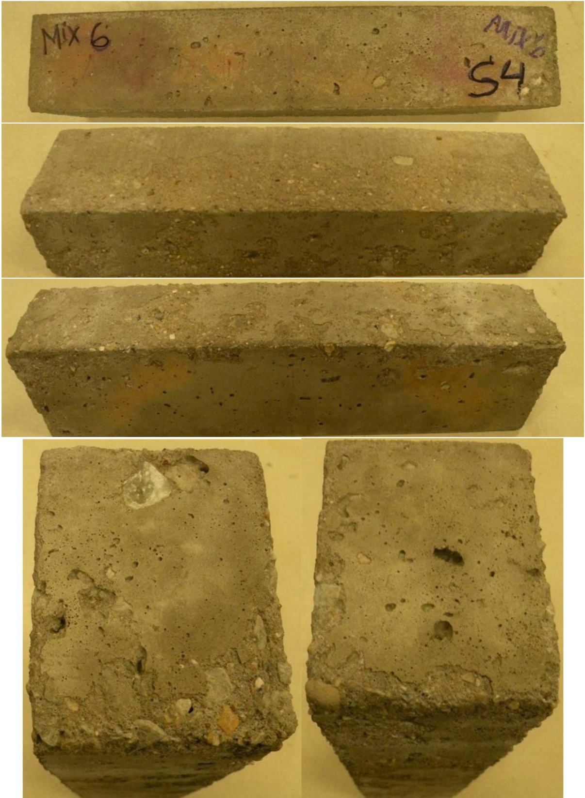
Figure O-17 Mix 6—Specimen #4 (DF= 96.49, Fresh Air = 8.1%, Hardened Entrained Air = 6.91%)
