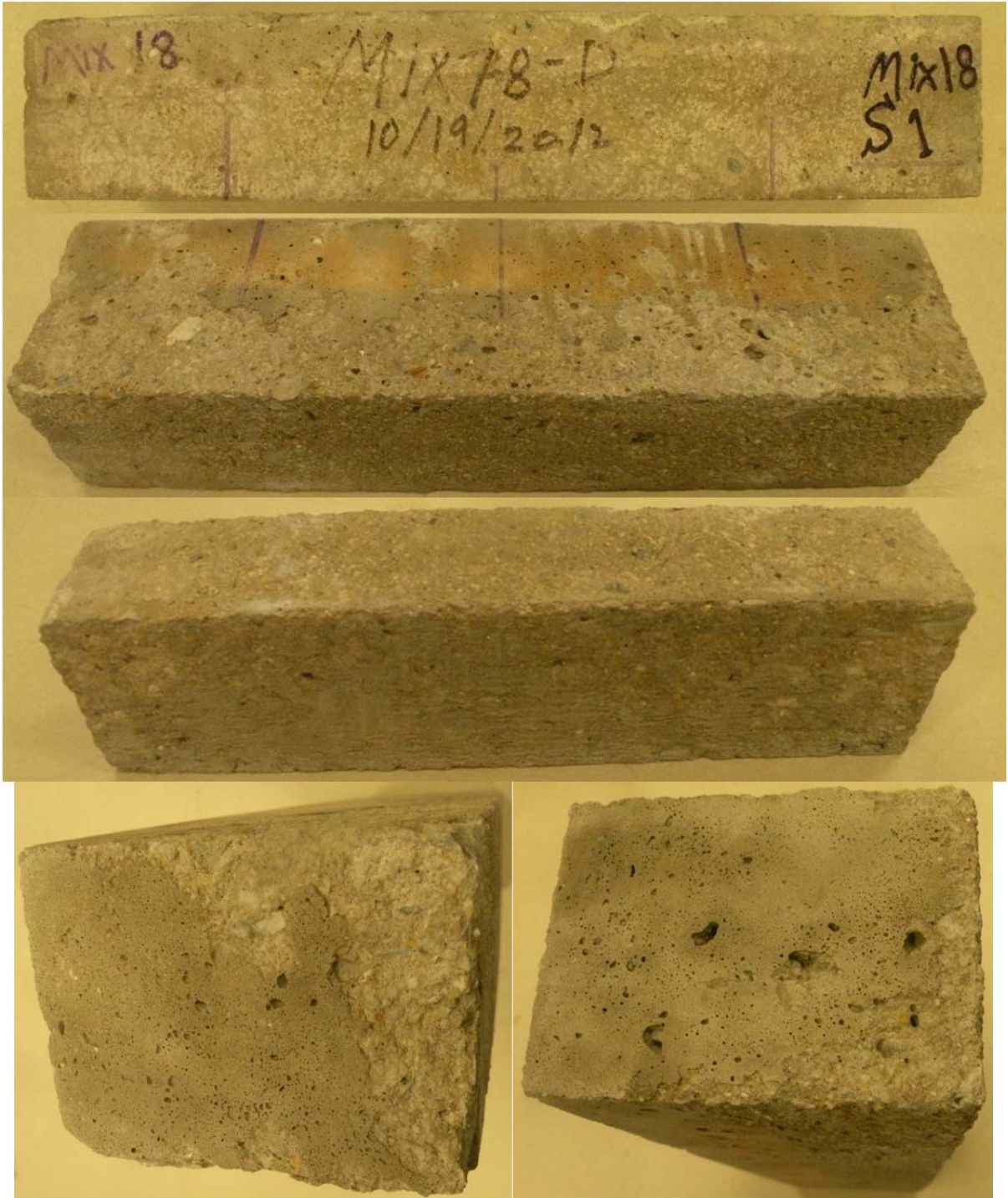
Figure O-40 Mix 18—Specimen #1 (DF = 94.67, Fresh Air = 8.0%, Hardened Entrained Air = 5.8%)
