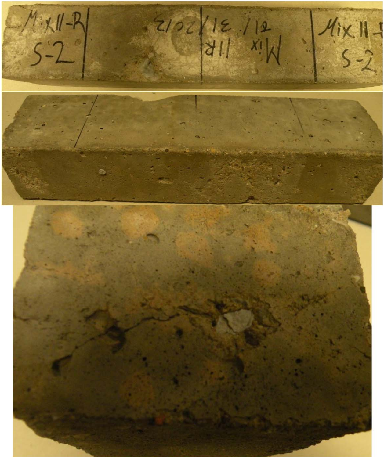
Figure O-32 Mix 11R—Specimen #2 (DF = 62.12, Fresh Air = 8.1%, Hardened Entrained Air = 7.17%)
