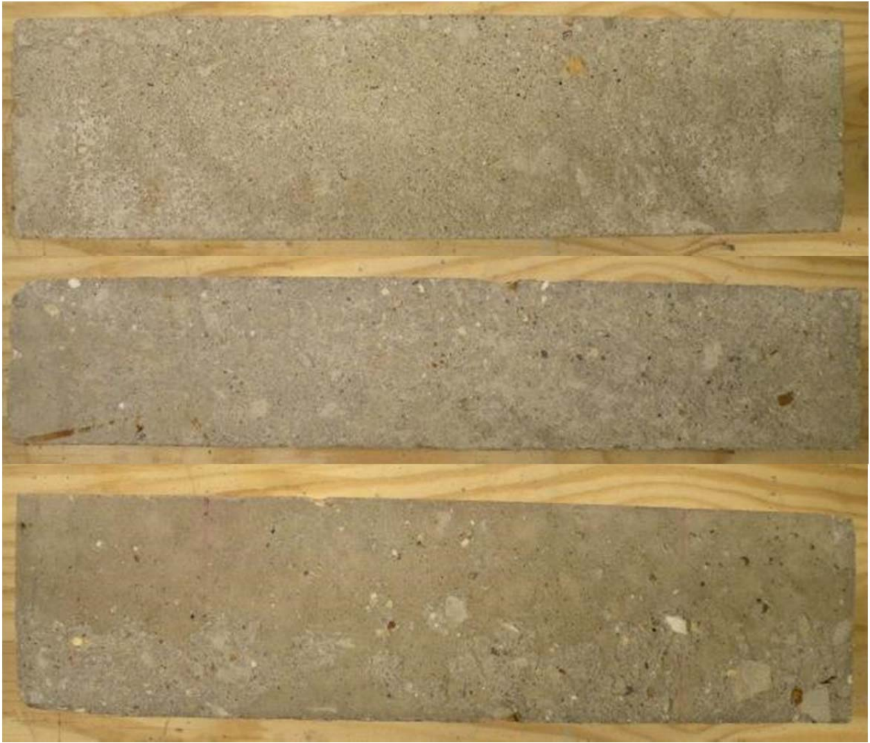
Figure O-21 Mix 9—Specimen #1 (DF = 59.31, Fresh Air = 6.6%, Hardened Entrained Air = 3.76%)
