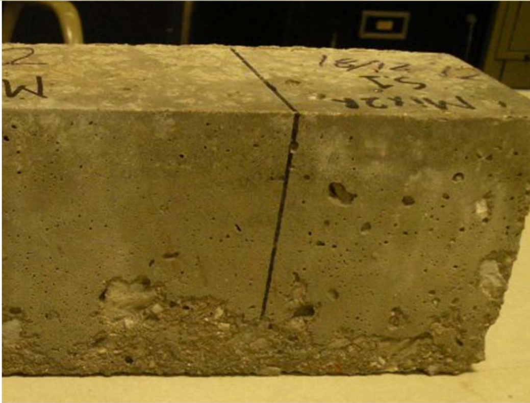
Figure O-10 Mix 2R–Specimen #1 (DF = 89.75, Fresh Air = 7.5%, Hardened Entrained Air = 7.26%)
