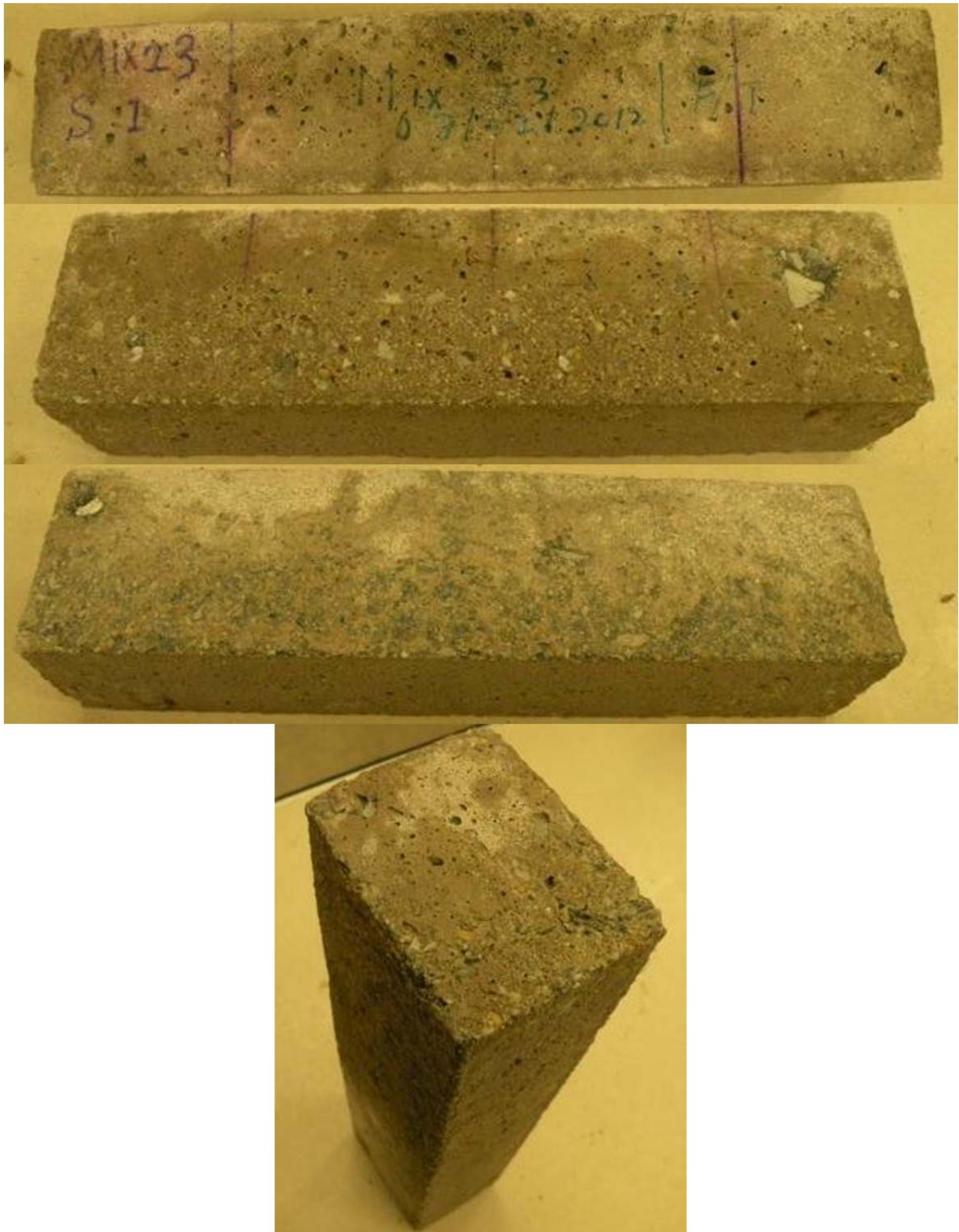
Figure O-47 Mix 23–Specimen #1 (DF = 78.45, Fresh Air = 7.8%, Hardened Entrained Air = 6.21%)
