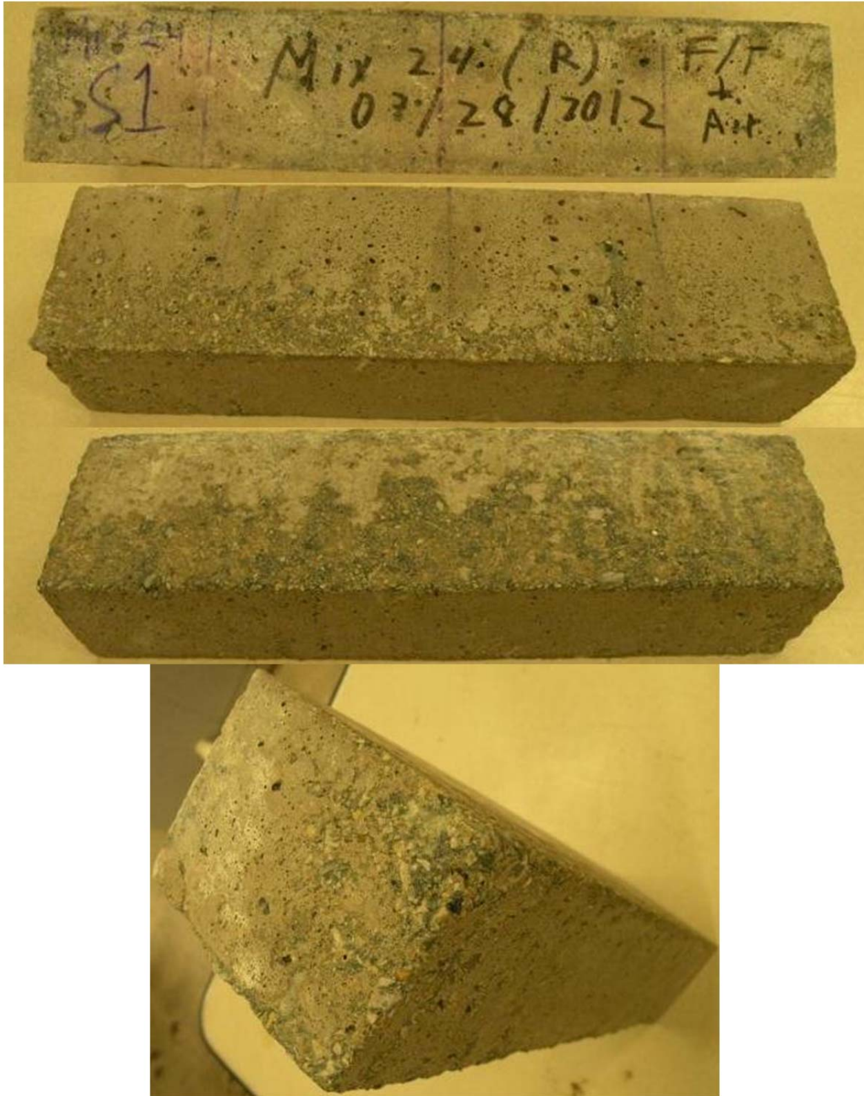
Figure O-49 Mix 24–Specimen #1 (DF = 91.35, Fresh Air = 7.3%, Hardened Entrained Air = 5.92%)
