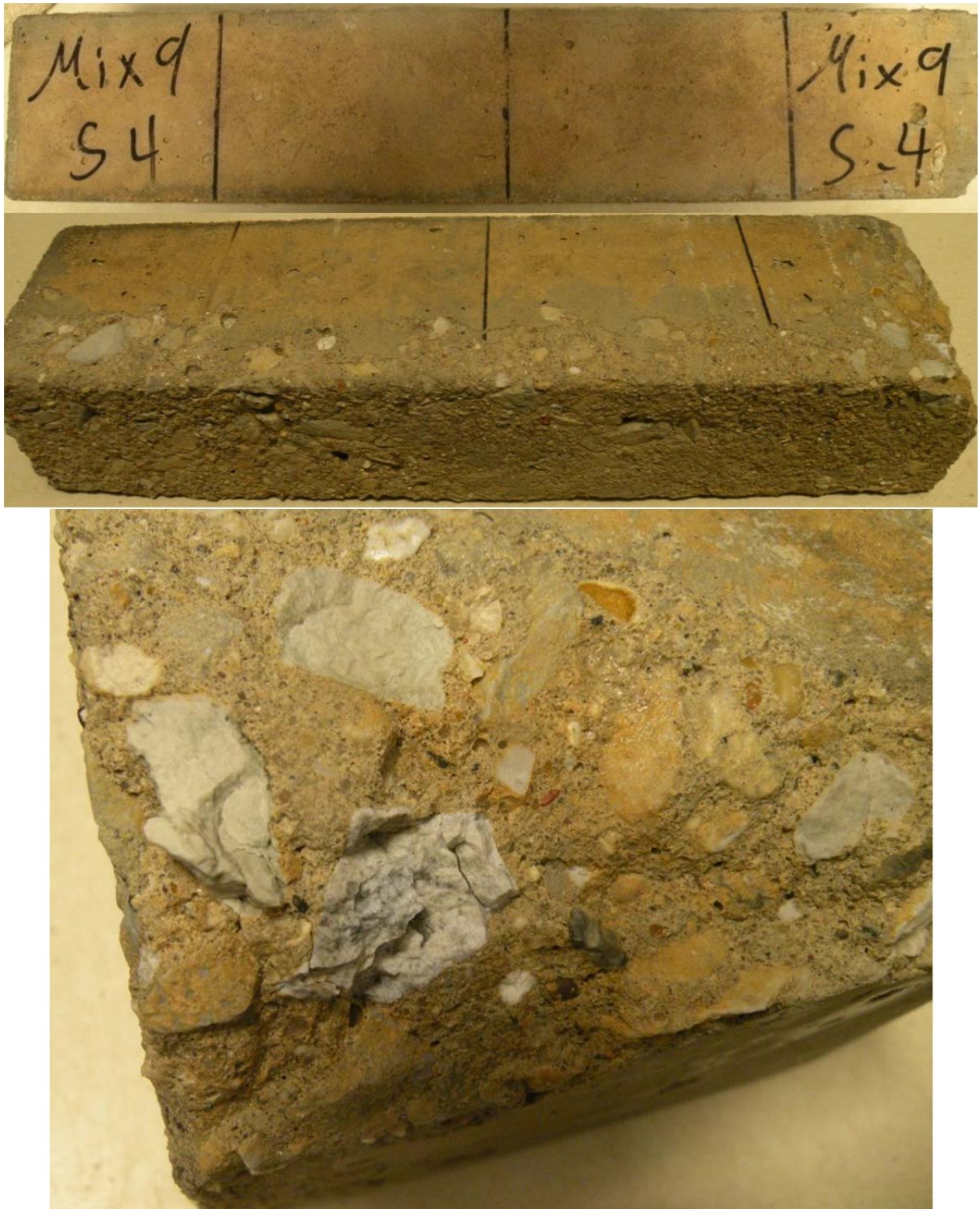
Figure O-29 Mix 9R–Specimen #4 (DF = 48.29, Fresh Air = 8%, Hardened Entrained Air = 5.29%)
