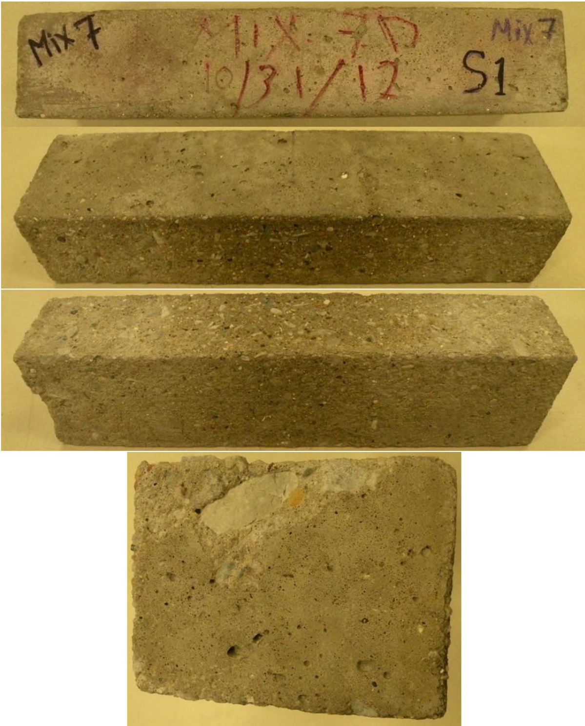
Figure O-18 Mix 7–Specimen #1 (DF= 91.49, Fresh Air = 8.0%, Hardened Entrained Air = 7.13%)
