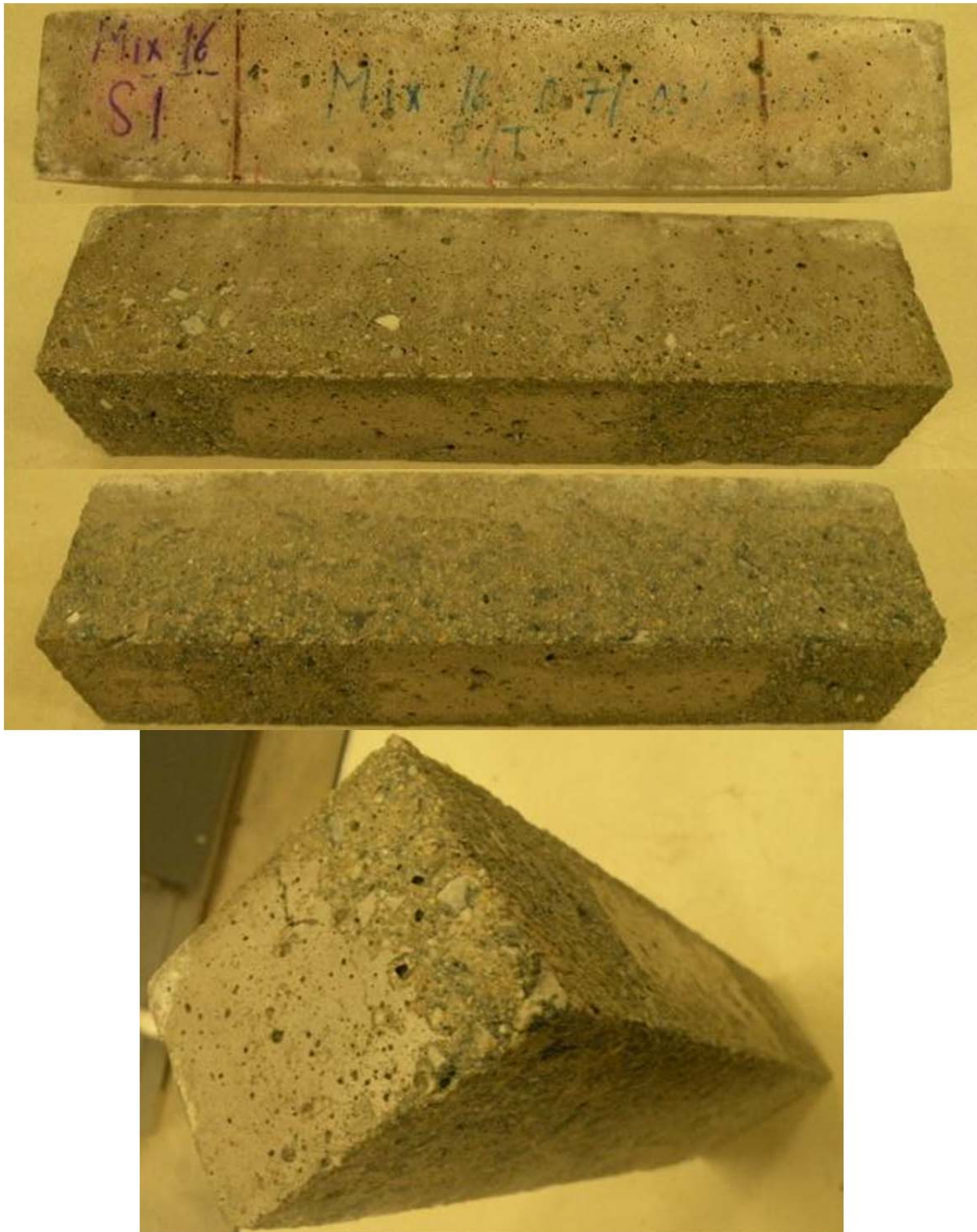
Figure O-37 Mix 16–Specimen #1 (DF = 77.47, Fresh Air = 6.9%, Hardened Entrained Air = 4.99%)
