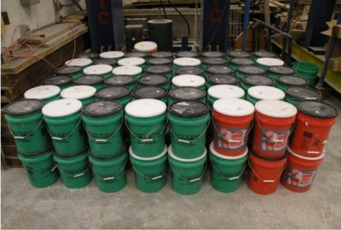
Figure 6-4 Aggregate stored in sealed buckets for maintaining the moisture content.
