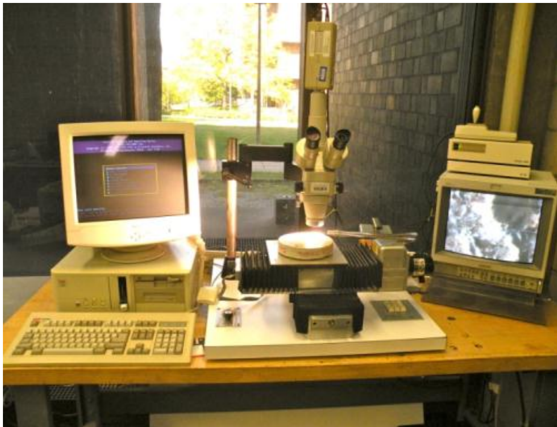
Figure 9-1 Microscopic determination of air void system parameters (ASTM C457).
