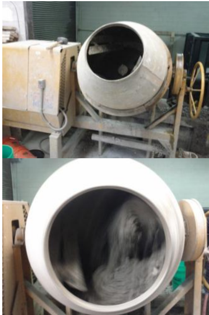
Figure 7-1 Concrete mixer (7 ft 3 capacity).
