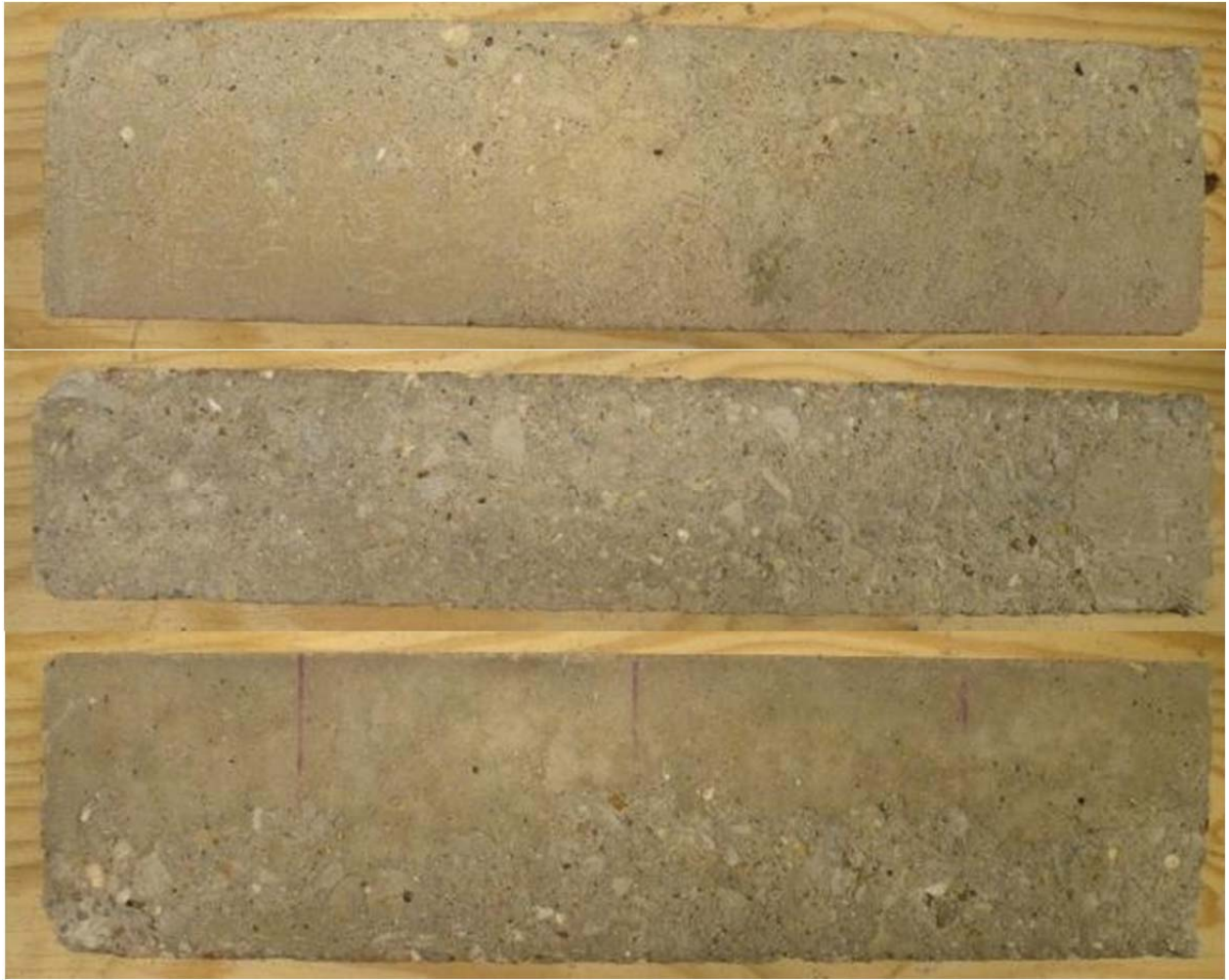
Figure O-24 Mix 10–Specimen #3 (DF = 50.62, Fresh Air = 6.5%, Hardened Entrained Air = 3.92%)
