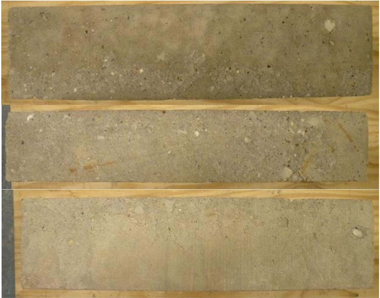
Figure O-22 Mix 9–Specimen #2 (DF = 66.09, Fresh Air = 6.6%, Hardened Entrained Air = 3.76%)
