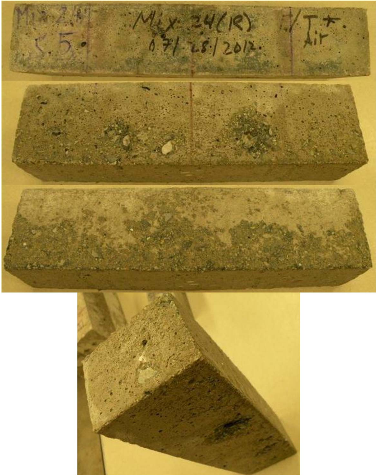
Figure O-50 Mix 24–Specimen #5 (DF = 76.37, Fresh Air = 7.3%, Hardened Entrained Air = 5.92%)
