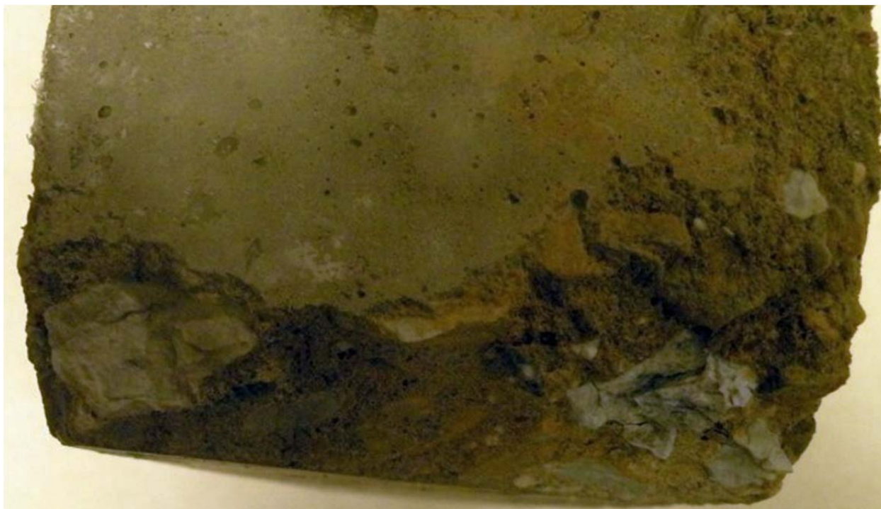
Figure O-29 (continued) Mix 9R–Specimen #4 (DF = 48.29, Fresh Air = 8%, Hardened Entrained Air = 5.29%)
