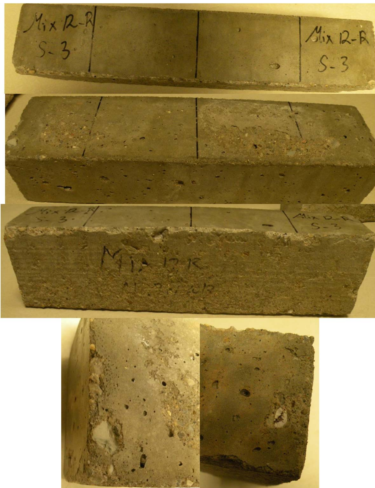
Figure O-33 Mix 12R—Specimen #3 (DF = 74.07, Fresh Air = 8%, Hardened Entrained Air = 5.75%)
