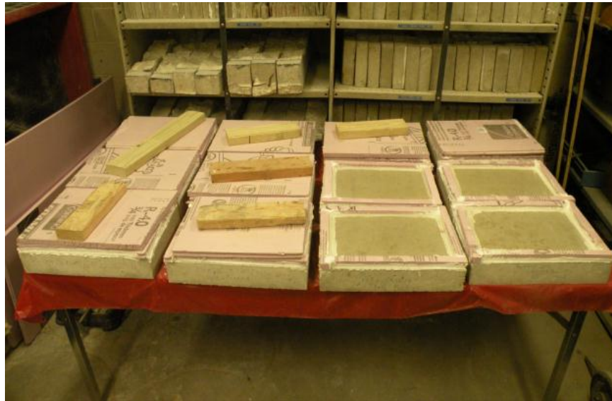
Figure 9-5 Salt ponding test, (chloride content across the slab depth).
