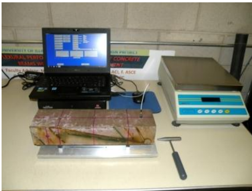
Figure 9-3 DK-5000 dynamic resonance frequency tester, ASTM C215.
