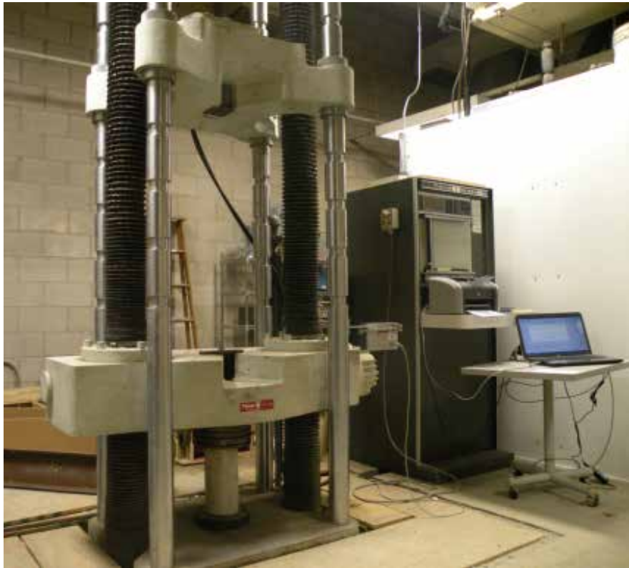
Figure 8-1 Test setup for compressive strength.
