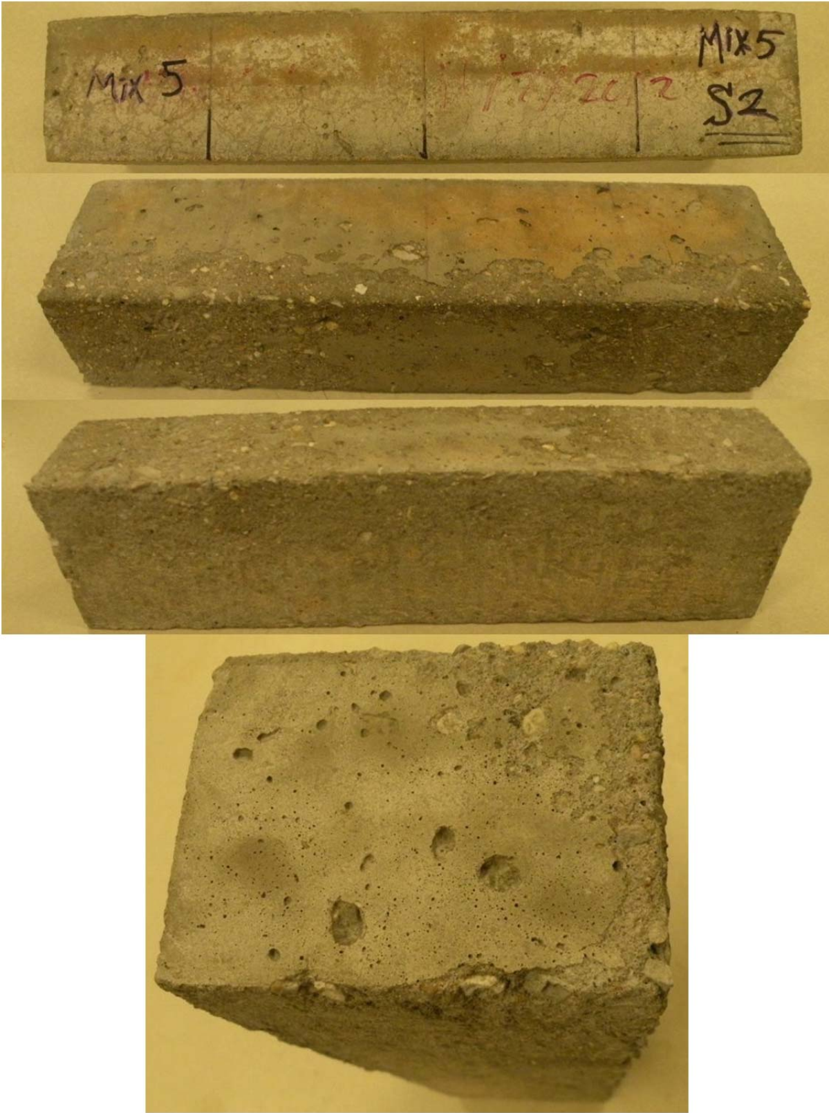
Figure O-14 Mix 5—Specimen #2 (DF = 94.85, Fresh Air = 7.9%, Hardened Entrained Air = 6.09%)
