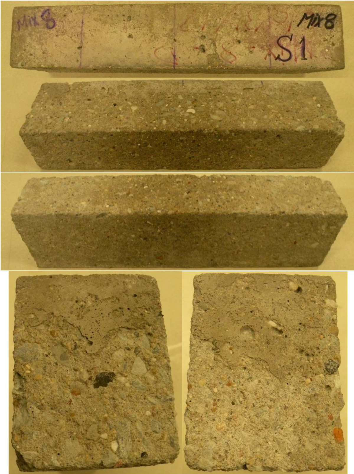
Figure O-20 Mix 8–Specimen #1 (DF = 88.2, Fresh Air = 8.0%, Hardened Entrained Air = 5.9%)
