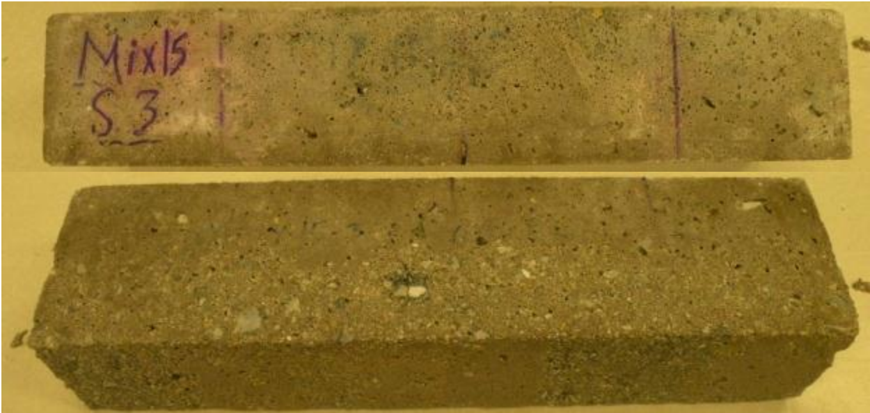
Figure 9-4 Mix15 Specimen #3 (DF = 64.63%, fresh air = 8%, hardened entrained air = 4.34%).
