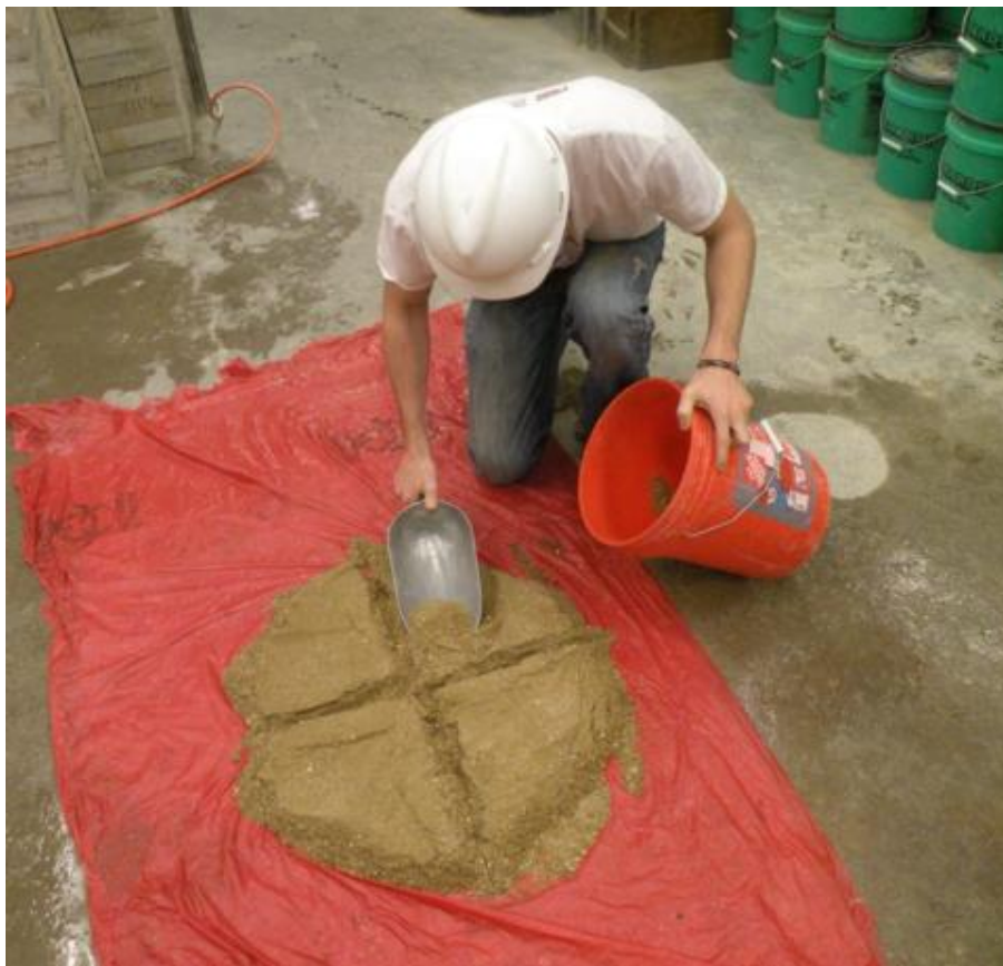
Figure 6-3 Quartering of fine aggregate for gradation sampling.
