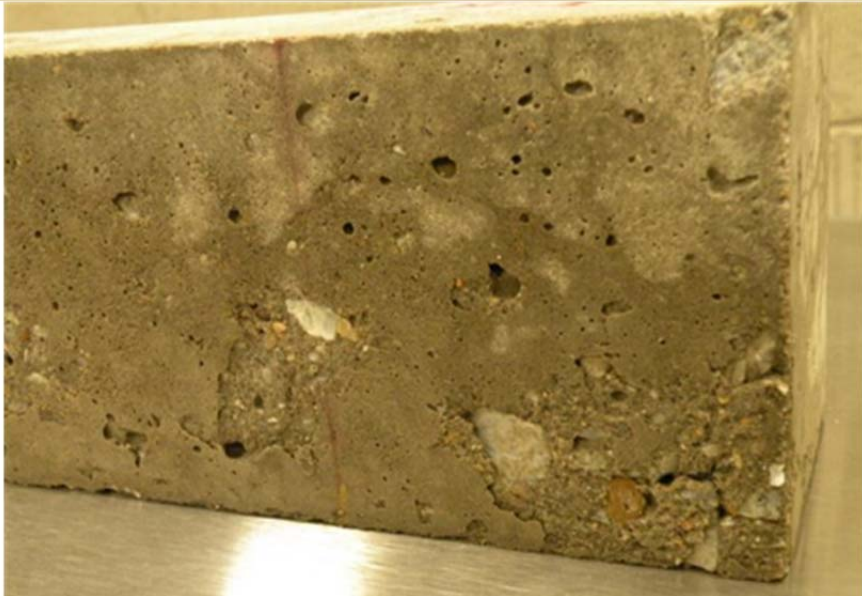
Figure O-27 Mix 12–Specimen #4 (DF = 84.31, Fresh Air = 6.3%, Hardened Entrained Air = 3.72%)
