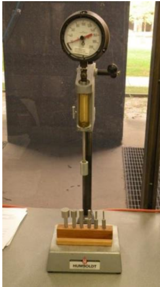
Figure 7-4 Penetration resistance testing equipment, ASTM C403.
