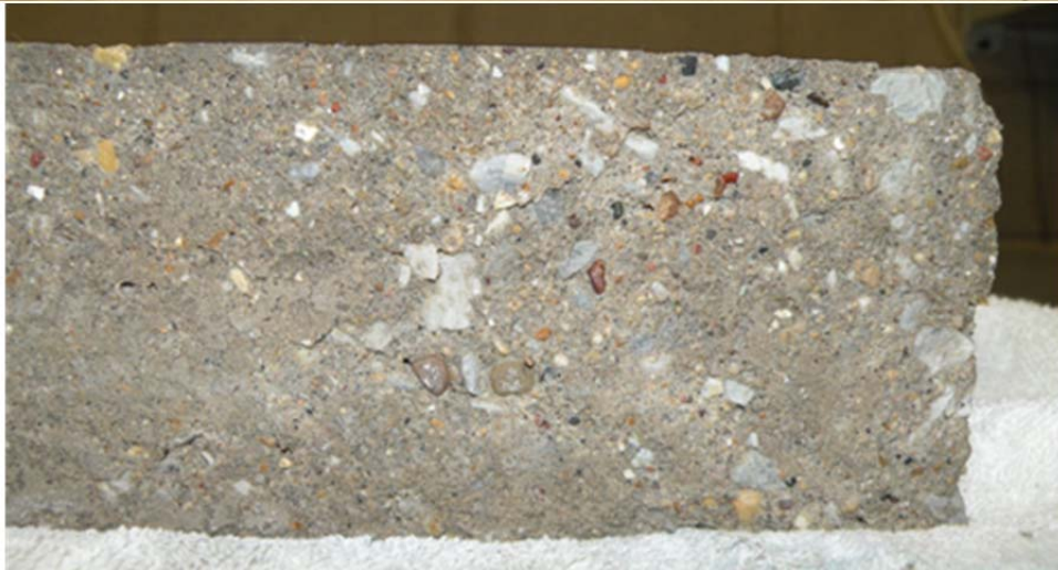
Figure O-23 Mix10–Specimen #2 (DF = 33.20, Fresh Air = 6.5%, Hardened Entrained Air = 3.92%)
