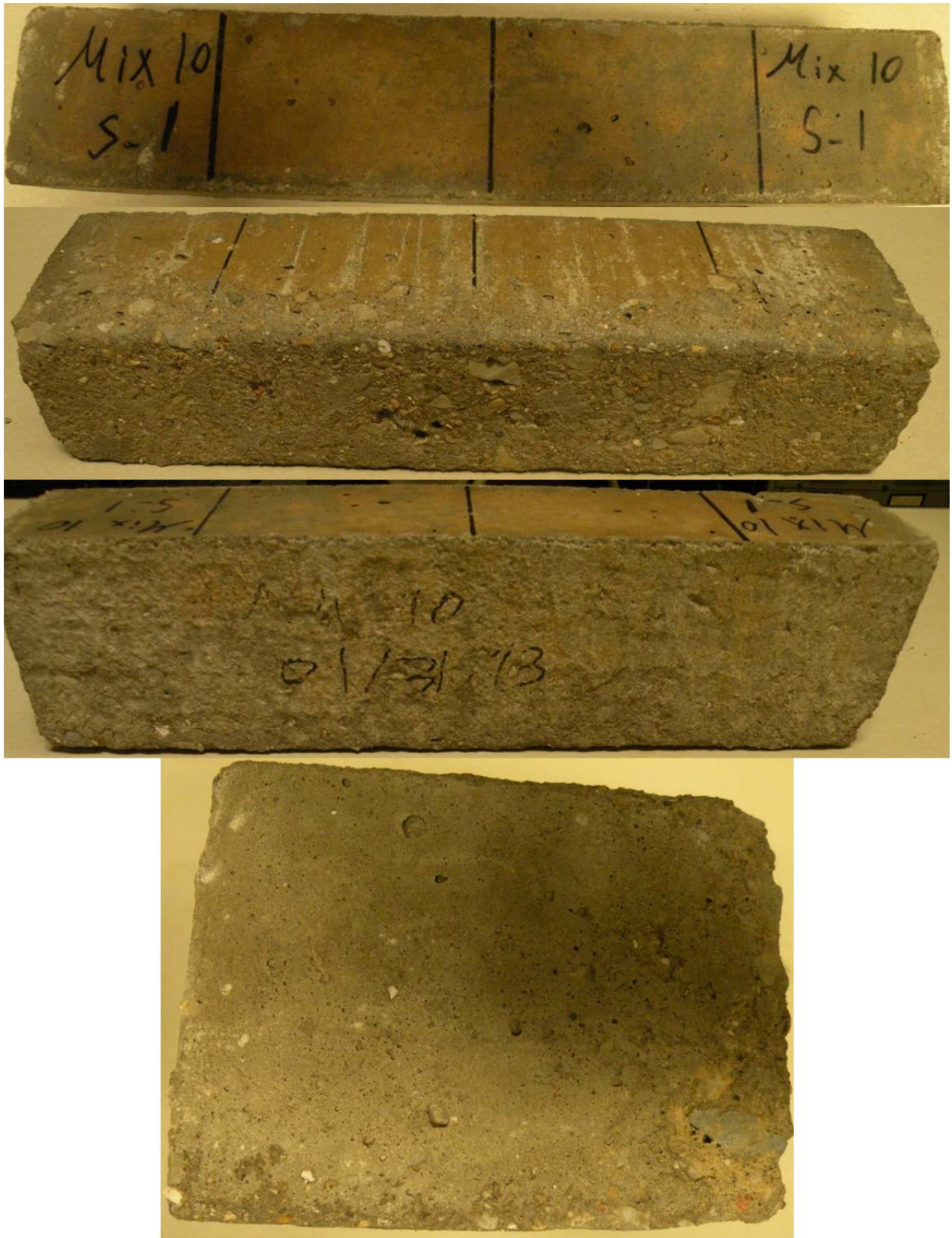
Figure O-30 Mix 10R–Specimen #1 (DF = 90.56, Fresh Air = 7.5%, Hardened Entrained Air = 4.5%)
