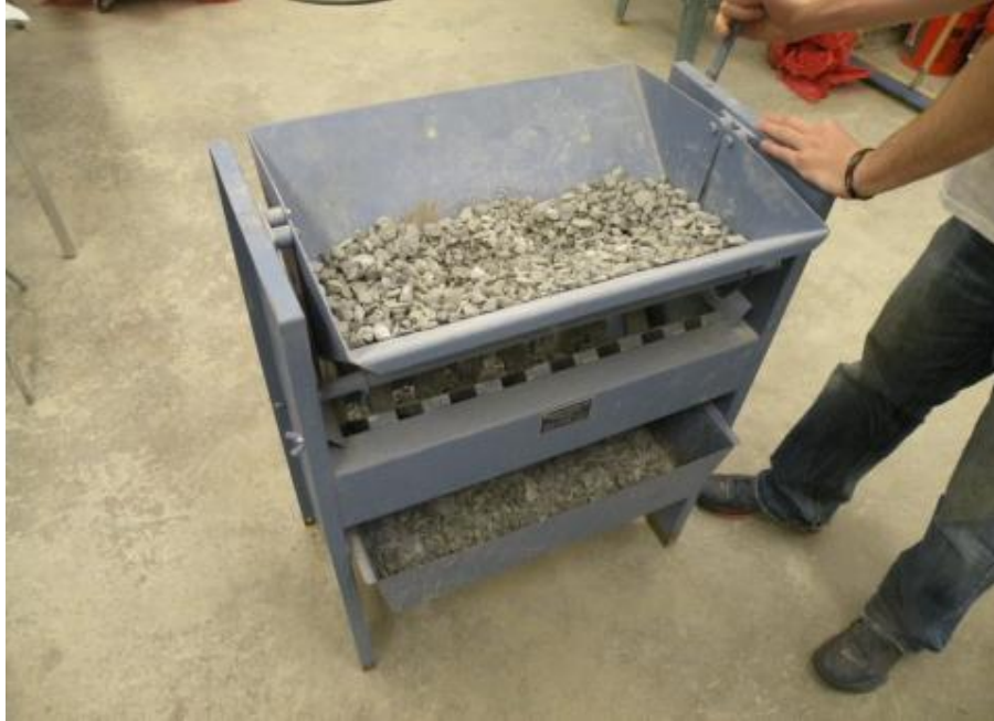
Figure 6-2 Mechanical splitting device for coarse aggregate gradation sampling.
