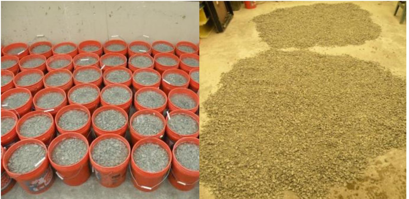
Figure 6-5 Coarse aggregate preparation for SSD condition.
