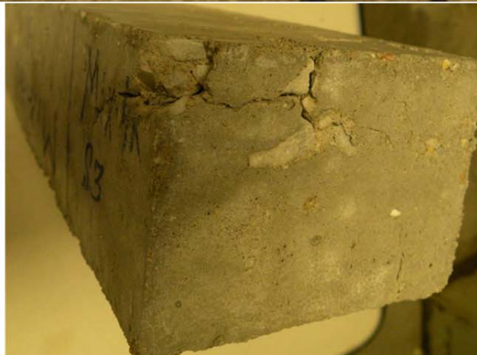
Figure O-13 Mix 4R–Specimen #3 (DF = 68.06, Fresh Air = 7.3%, Hardened Entrained Air = 7.92%)
