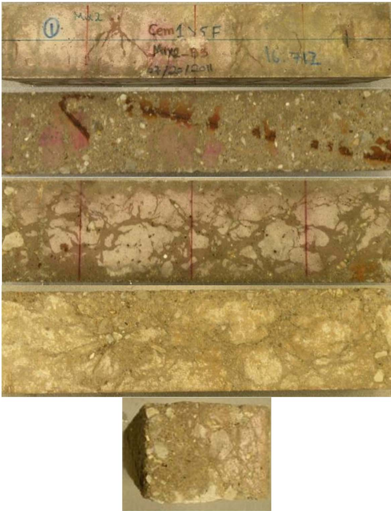
Figure O-2 Mix 2–Specimen #1 (DF = 50.06, Fresh Air = 7%, Hardened Entrained Air = 3.03%)
