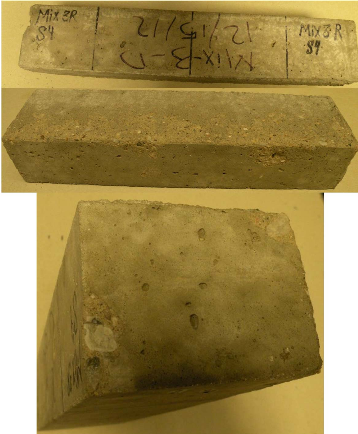
Figure O-12 Mix 3R–Specimen #4 (DF = 85.21, Fresh Air = 7.5%, Hardened Entrained Air = 7.47%)
