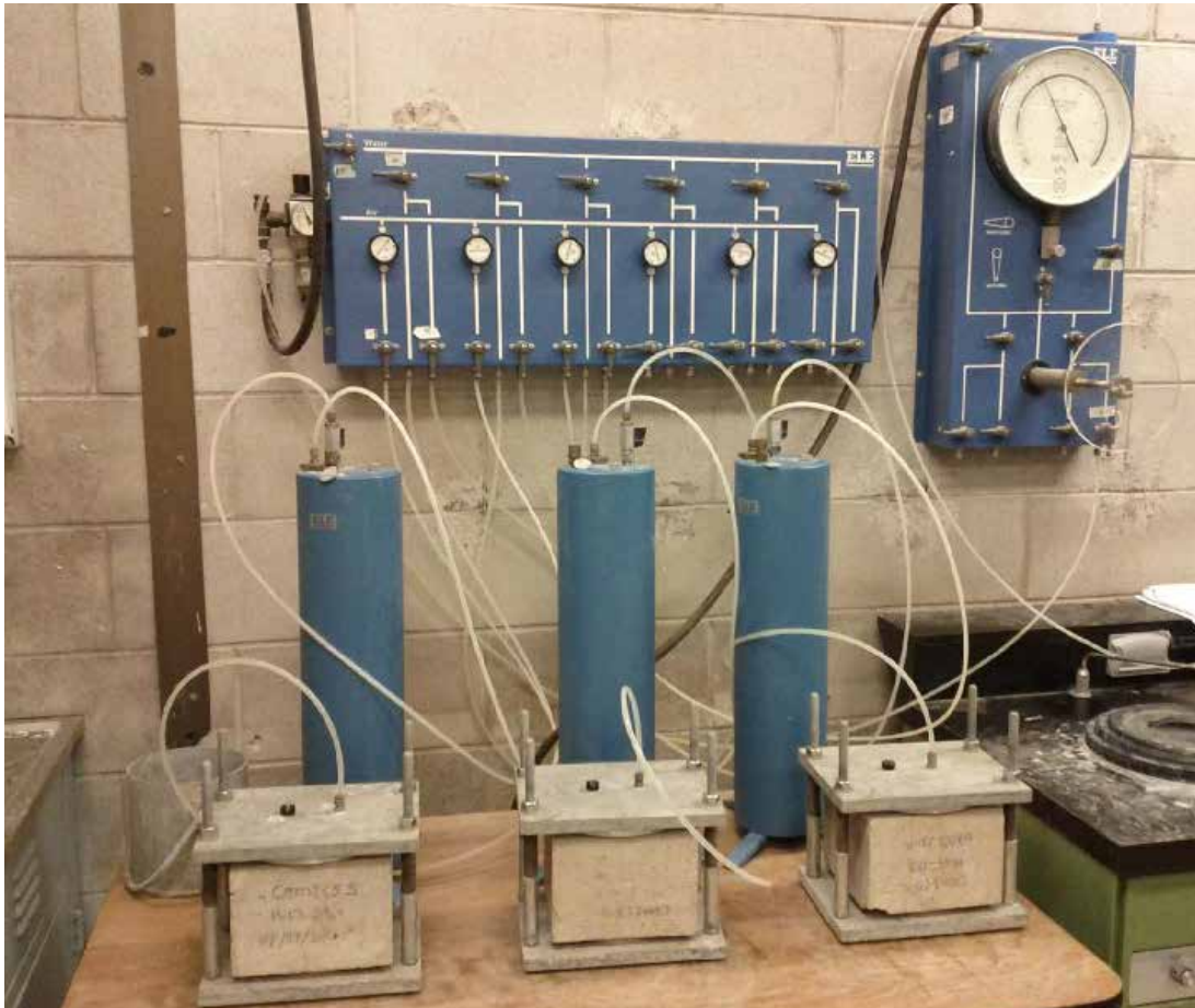
Figure 9-15 Water permeability test setup, DIN 1048.
