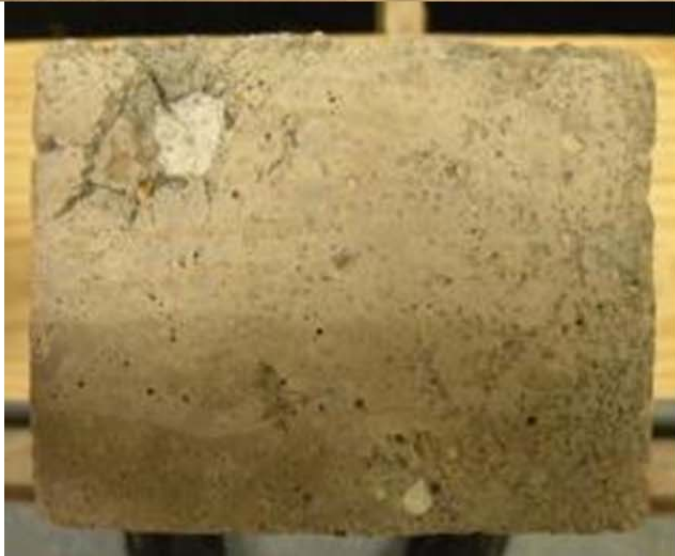
Figure O-25 Mix 11—Specimen #4 (DF = 87.04, Fresh Air = 6.6%, Hardened Entrained Air = 3.90%)
