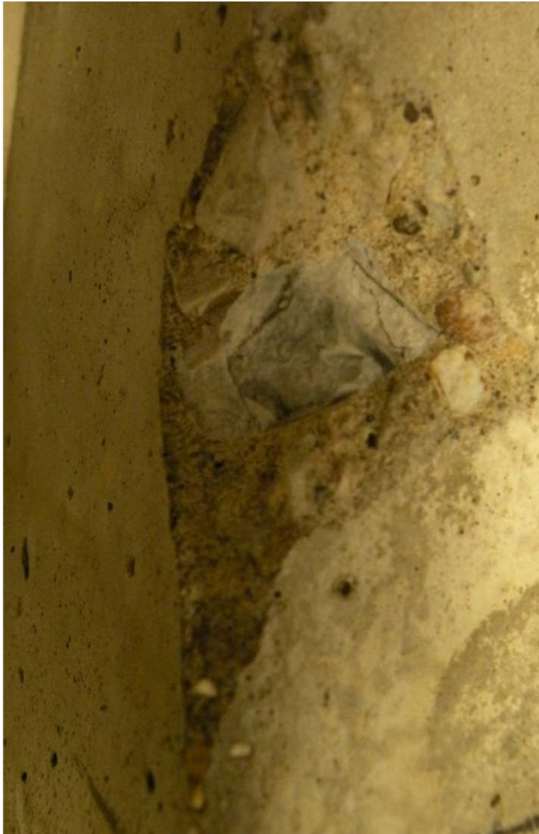
Figure O-32 (continued) Mix 11R–Specimen #2 (DF = 62.12, Fresh Air = 8.1%, Hardened Entrained Air = 7.17%)
