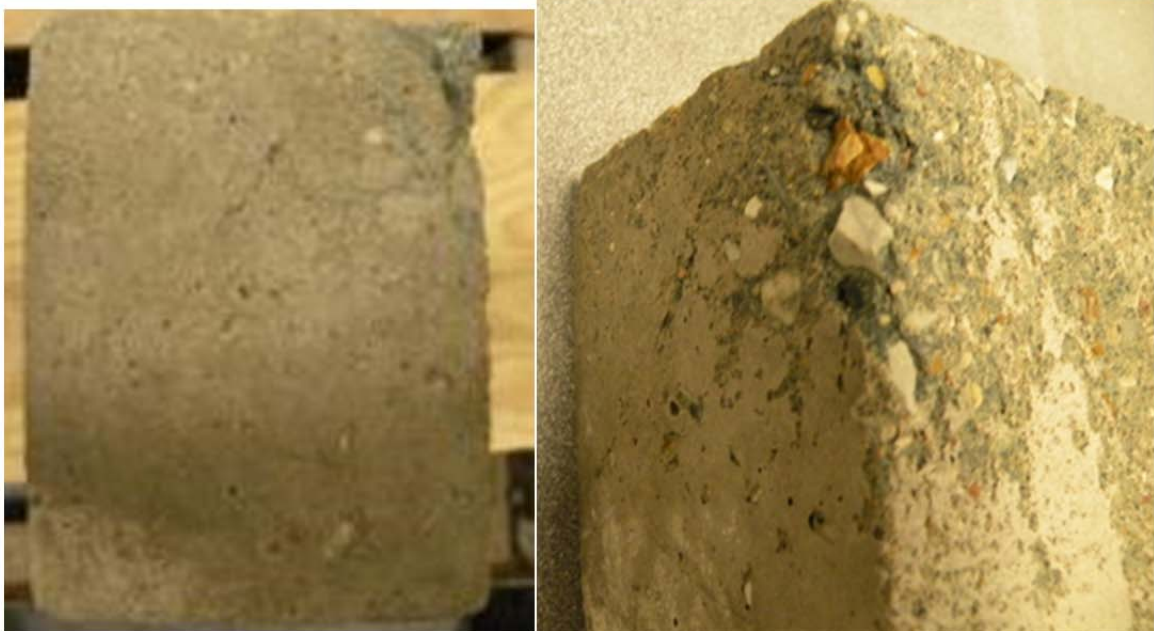
Figure O-26 Mix12–Specimen #3 (DF = 39.33, Fresh Air = 6.3%, Hardened Entrained Air = 3.72%)
