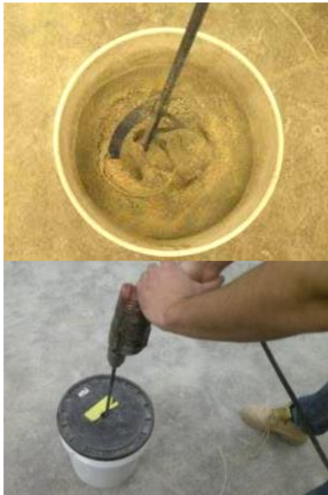
Figure 6-1 Preparing Cem2 by blending Cem1R with fly ash.
