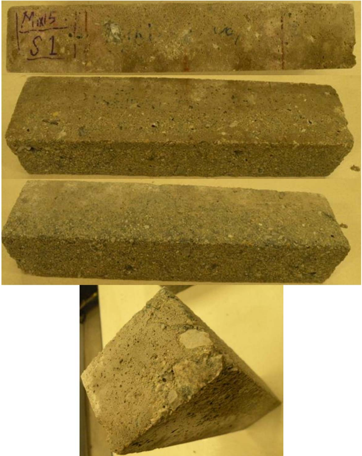
Figure O-36 Mix 15—Specimen #1 (DF = 45.59, Fresh Air = 8.1%, Hardened Entrained Air = 4.34%)
