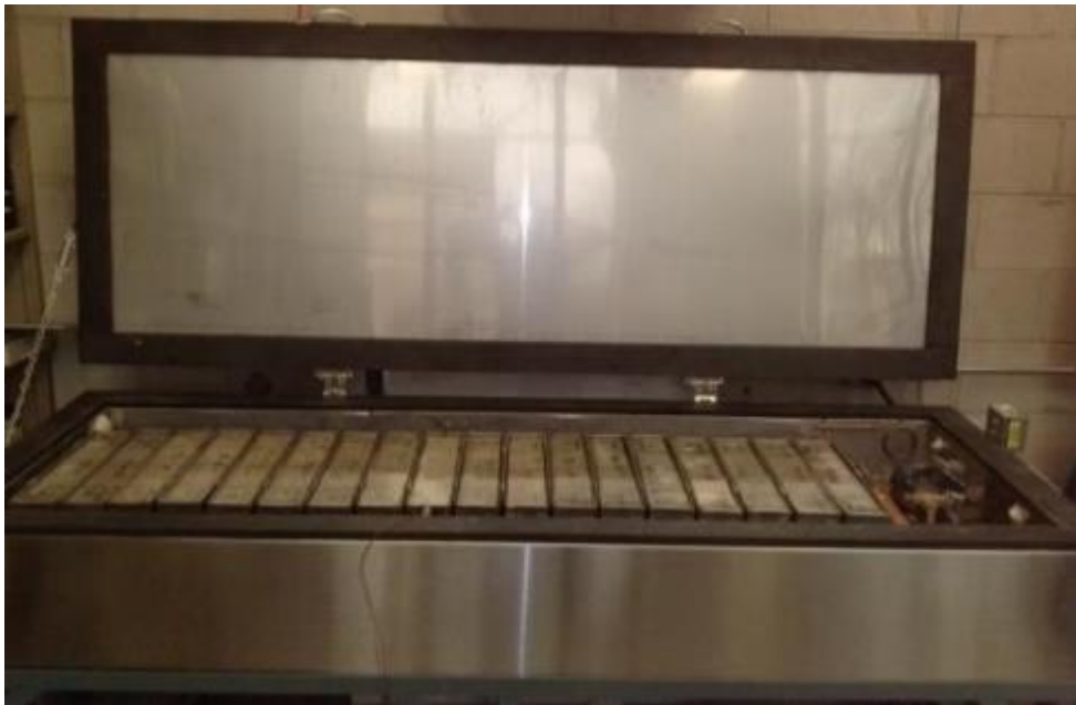
Figure 9-2 Freeze/thaw test cabinet, ASTM C666, procedure A.
