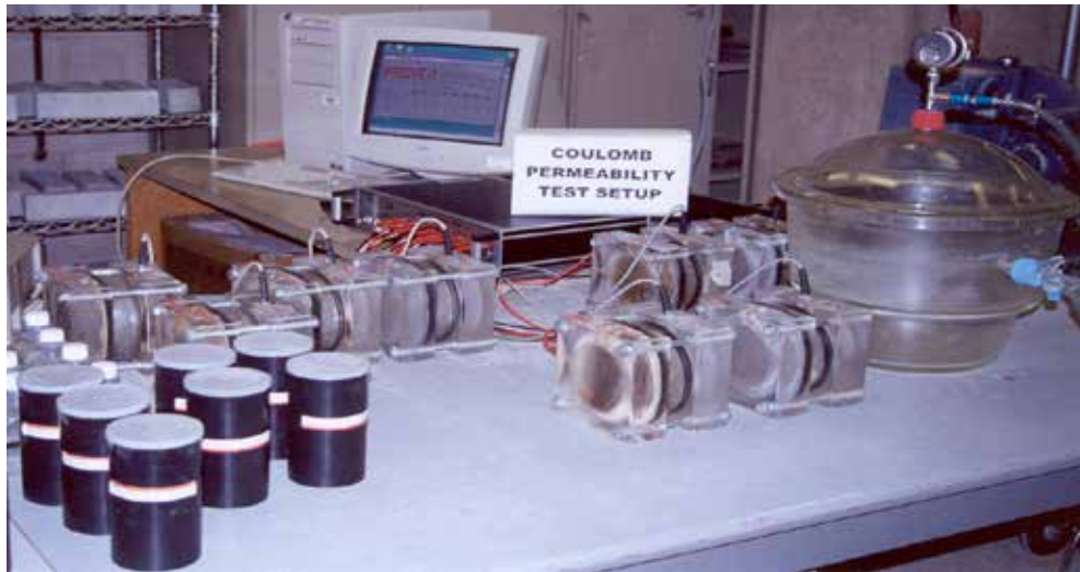
Figure 9-19 Rapid chloride permeability test, ASTM C1202/AASHTO T277.
