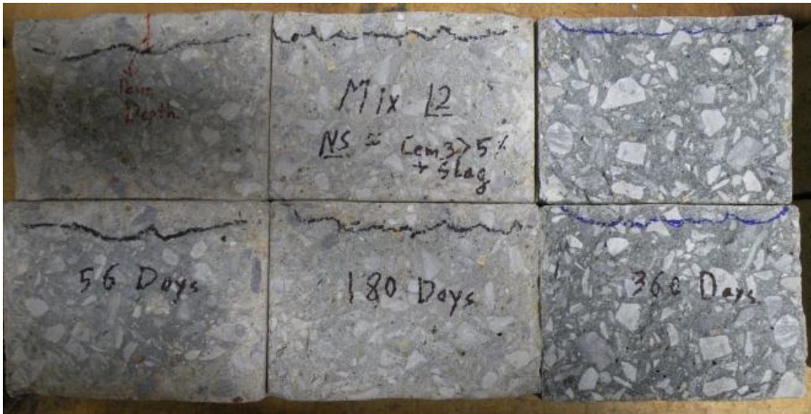
Figure 9-16 Depth of penetration in Mix 12 specimens.
