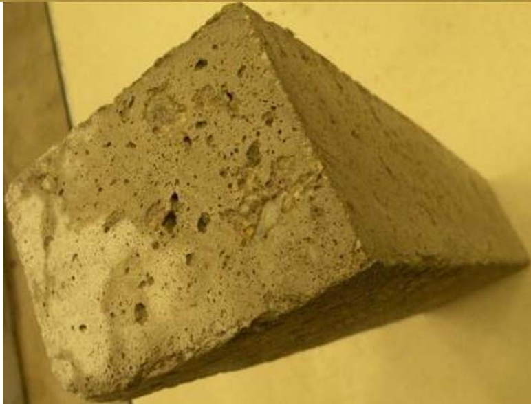
Figure O-45 Mix 22–Specimen #3 (DF = 89.66, Fresh Air = 7.2%, Hardened Entrained Air = 6.46%)
