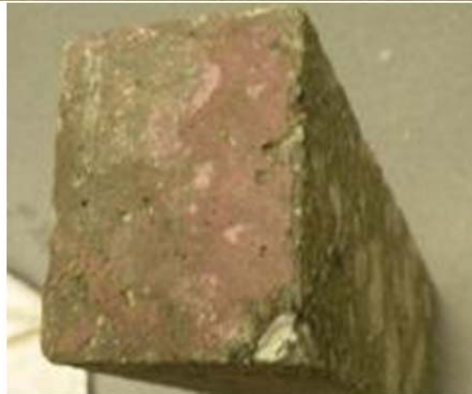
Figure O-5 Mix3-Specimen #4 (DF = 57.94, Fresh Air = 6.5%, Hardened Entrained Air = 4.06%)
