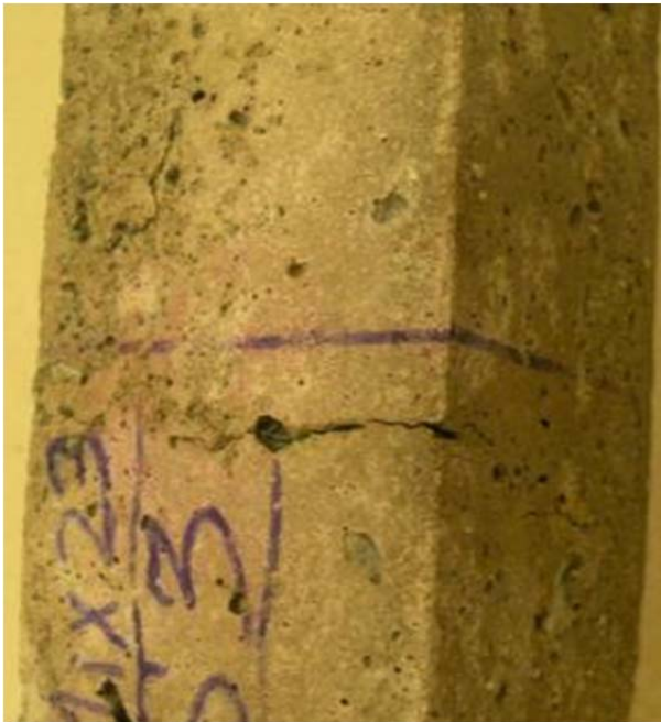
Figure O-48 Mix 23–Specimen #3 (DF = 24.06, Fresh Air = 7.8%, Hardened Entrained Air = 6.21%)
