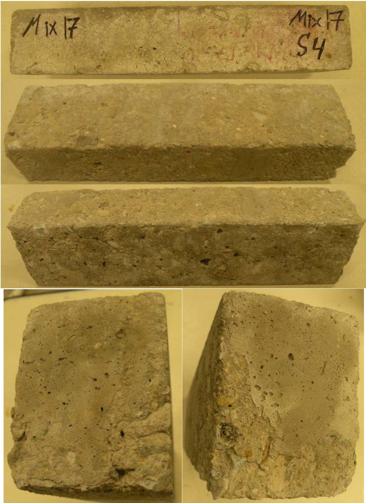
Figure O-39 Mix 17–Specimen #4 (DF= 92.86, Fresh Air = 7.9%, Hardened Entrained Air = 5.95%)
