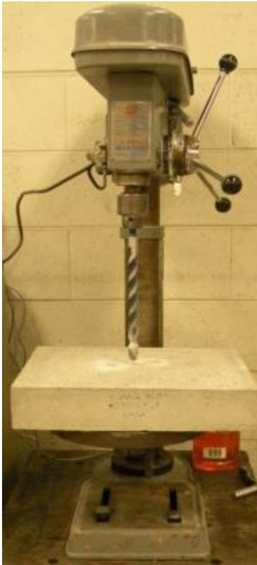
Figure 9-6 Drilling press used to collect powdered concrete samples.
