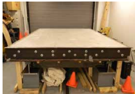
Figure 23. Concrete deck after the pour.
