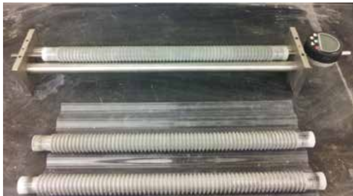
Figure A.2. A dilatometer for monitoring the unrestrained deformation of cement pastes according to ASTM C1698.
