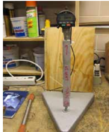
Figure A.3. Typical mortar sample and digital length comparator for free shrinkage measurement.
