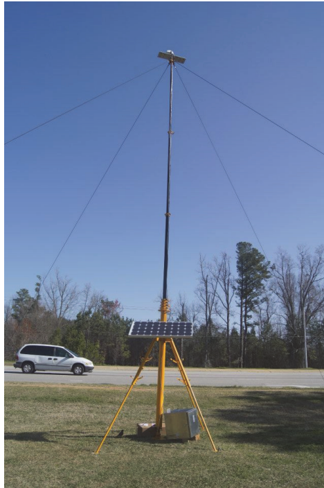
Figure 4-13 RTMS Field Installation
